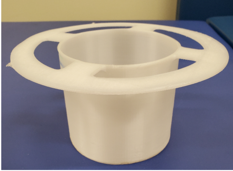
Figure 5.8: The fabricated cylindrical phantom used in the image noise measurements.
