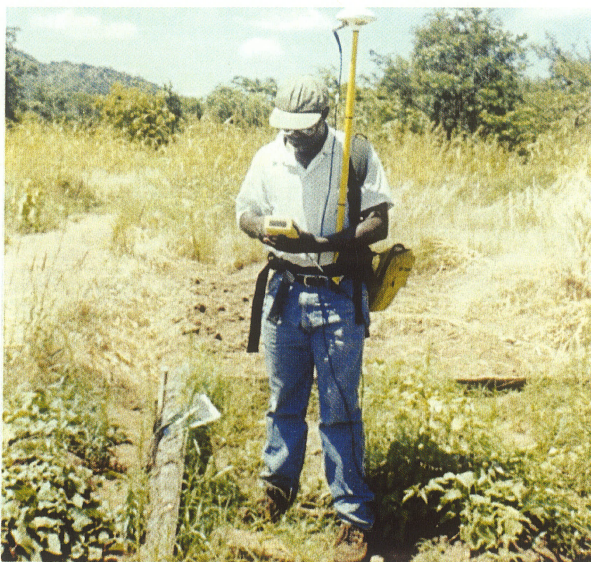
Fig. 5.5: Determining coordinates of a validation plot using differential GPS
