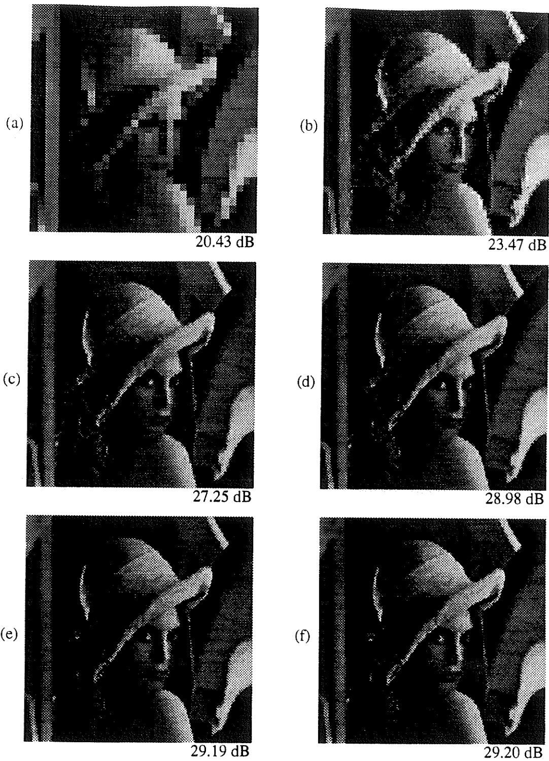
Fig. 8.3. The first six iterations of the fractal image reconstruction procedure. Images are displayed at 60% of their actual size.
