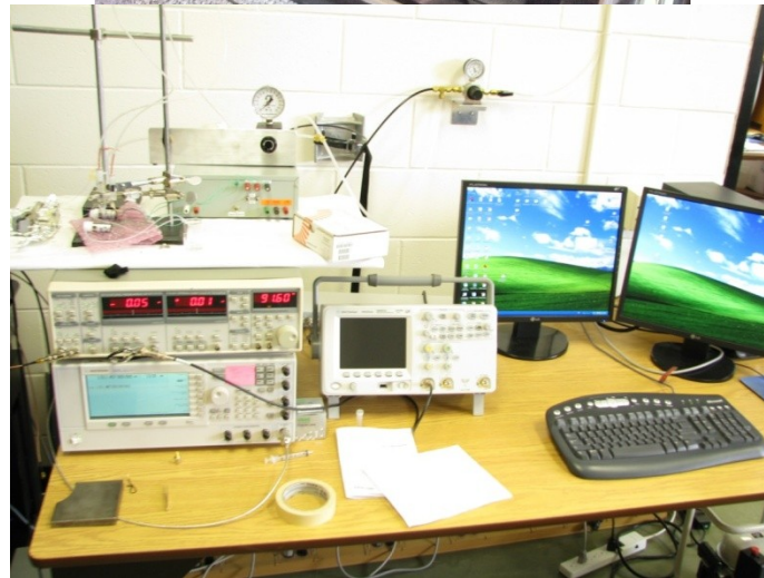
Figure 3-4: Microwave interferometer, resonant sensor, microfluidic device, and microscope located inside an EMI enclosure (top). Signal source, LIA, syringe apparatus, and computer interface (bottom).
