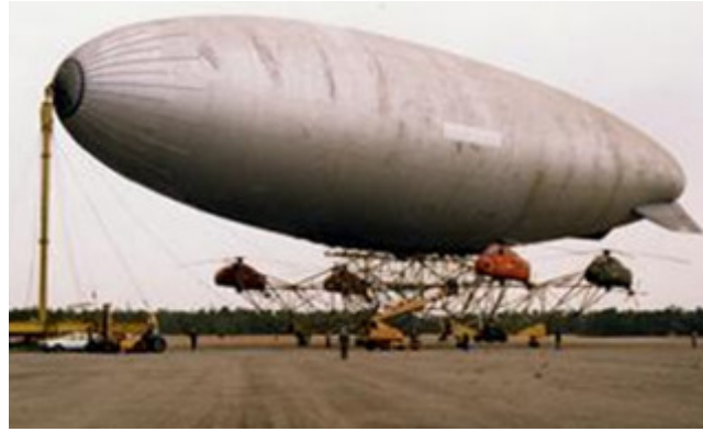
Figure 3: Piasecki PA-97 Helistat
