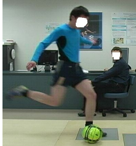
Figure 5. Ground reaction force data collection at Pan Am Biomechanics Lab.
