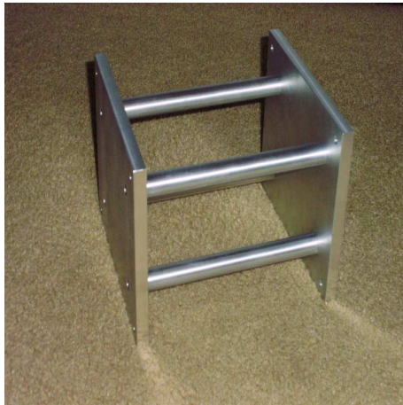
(a) The extension stage built to mount the scanner detector 18.5 cm upstream of the main detector.
