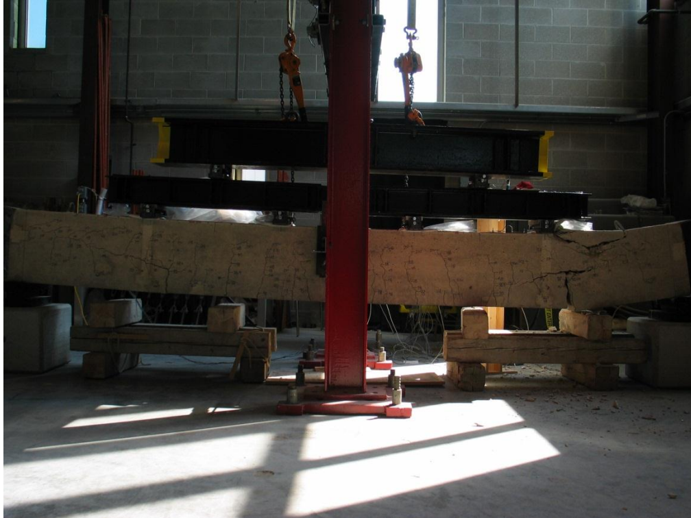
Figure 5.61 – RB2 right after final failure
