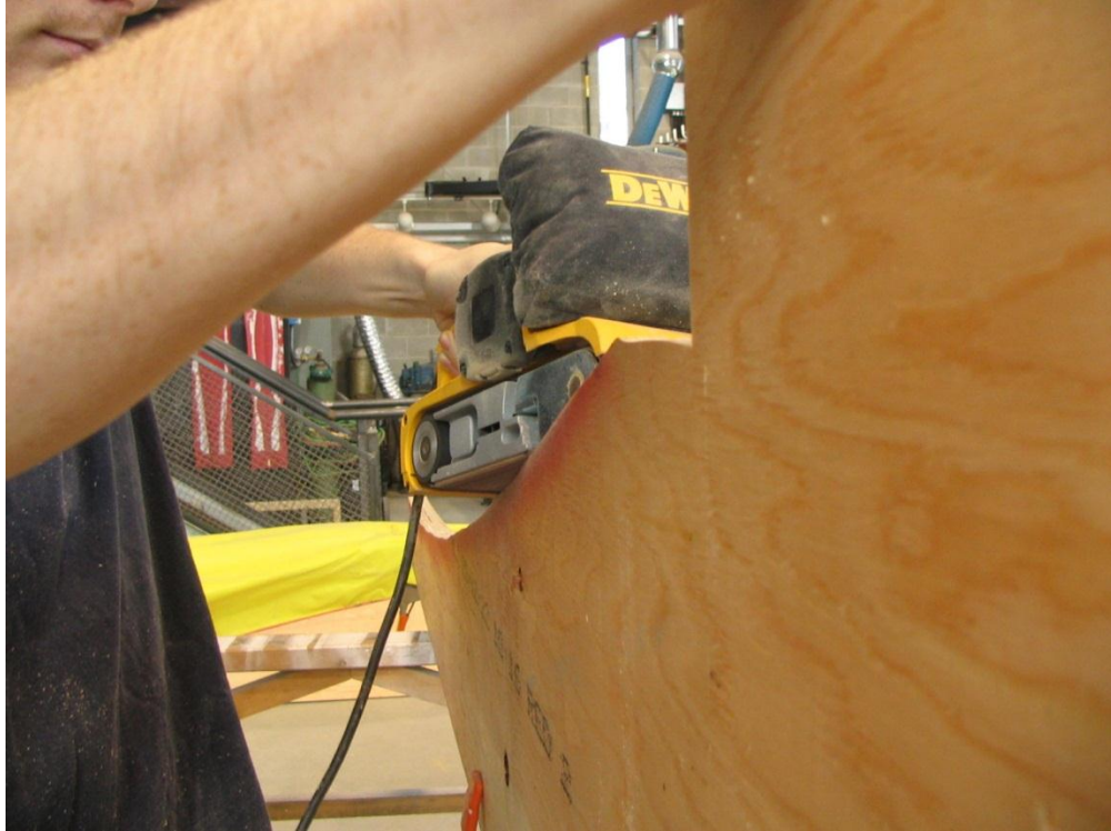
Figure 4.9 – Fairing of the curve
