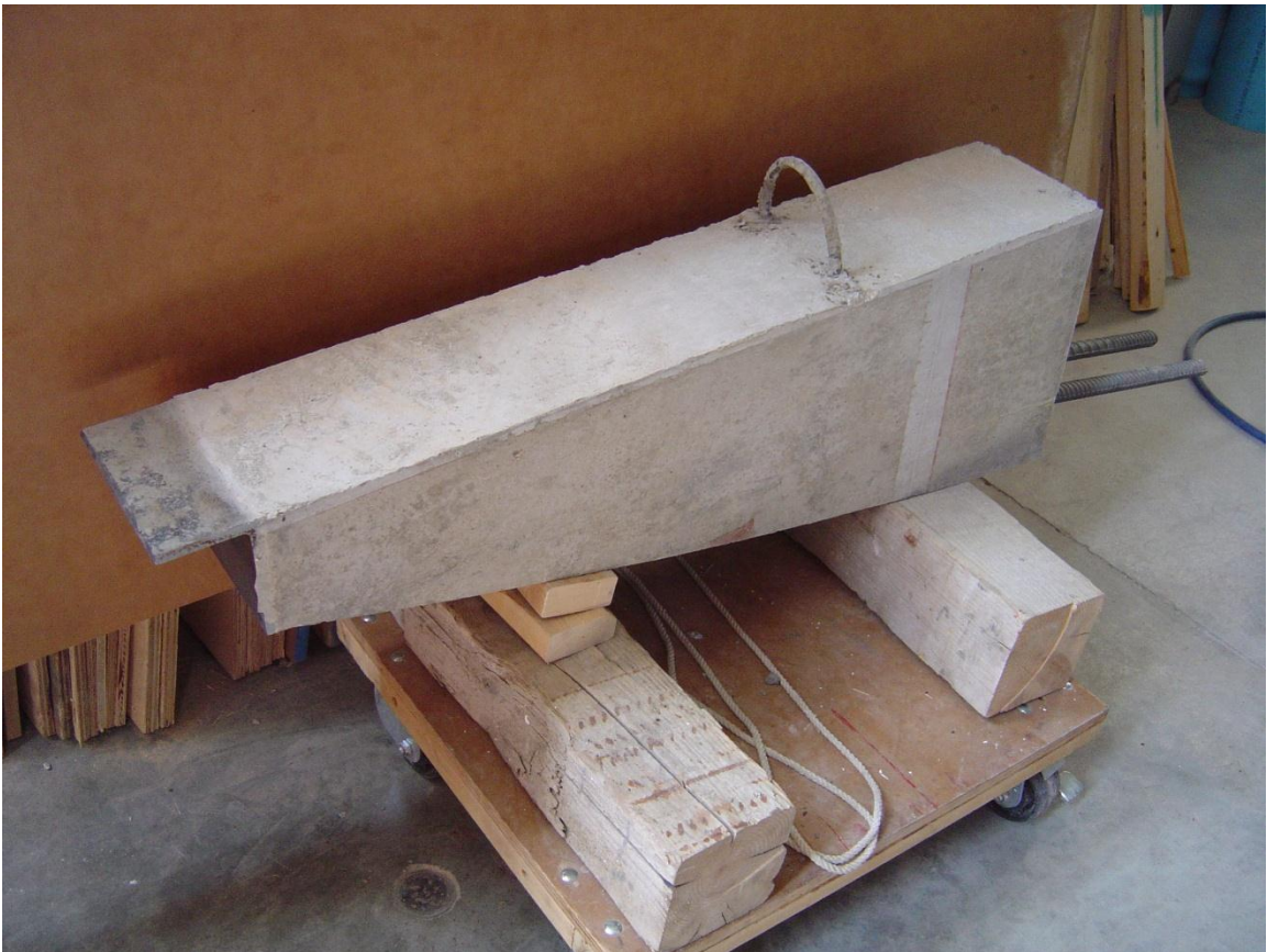
Figure 5.87 – ECB-RA1 prior to testing, showing the end angle reversed
