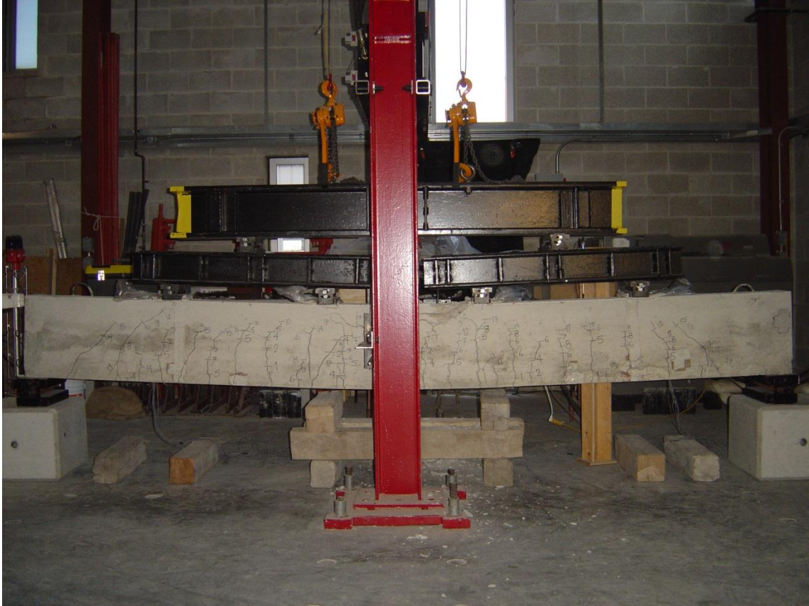
Figure 5.72 – RB3 right after failure
