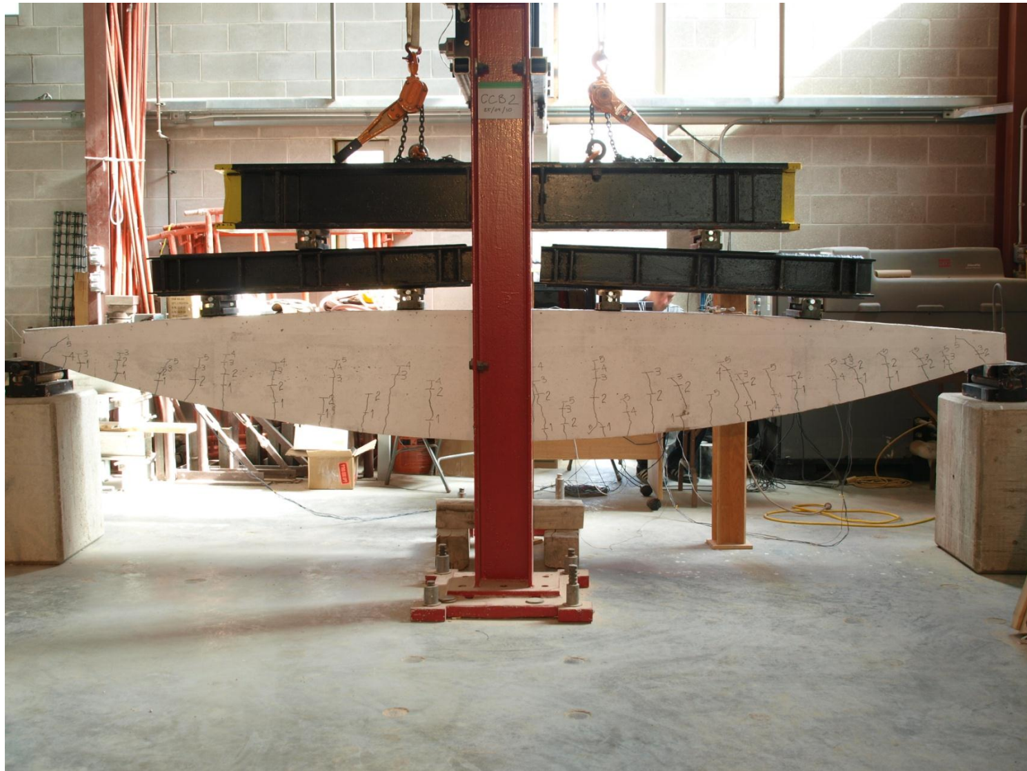
Figure 5.112 – CCB2 – Crack propagation at 130 kN
