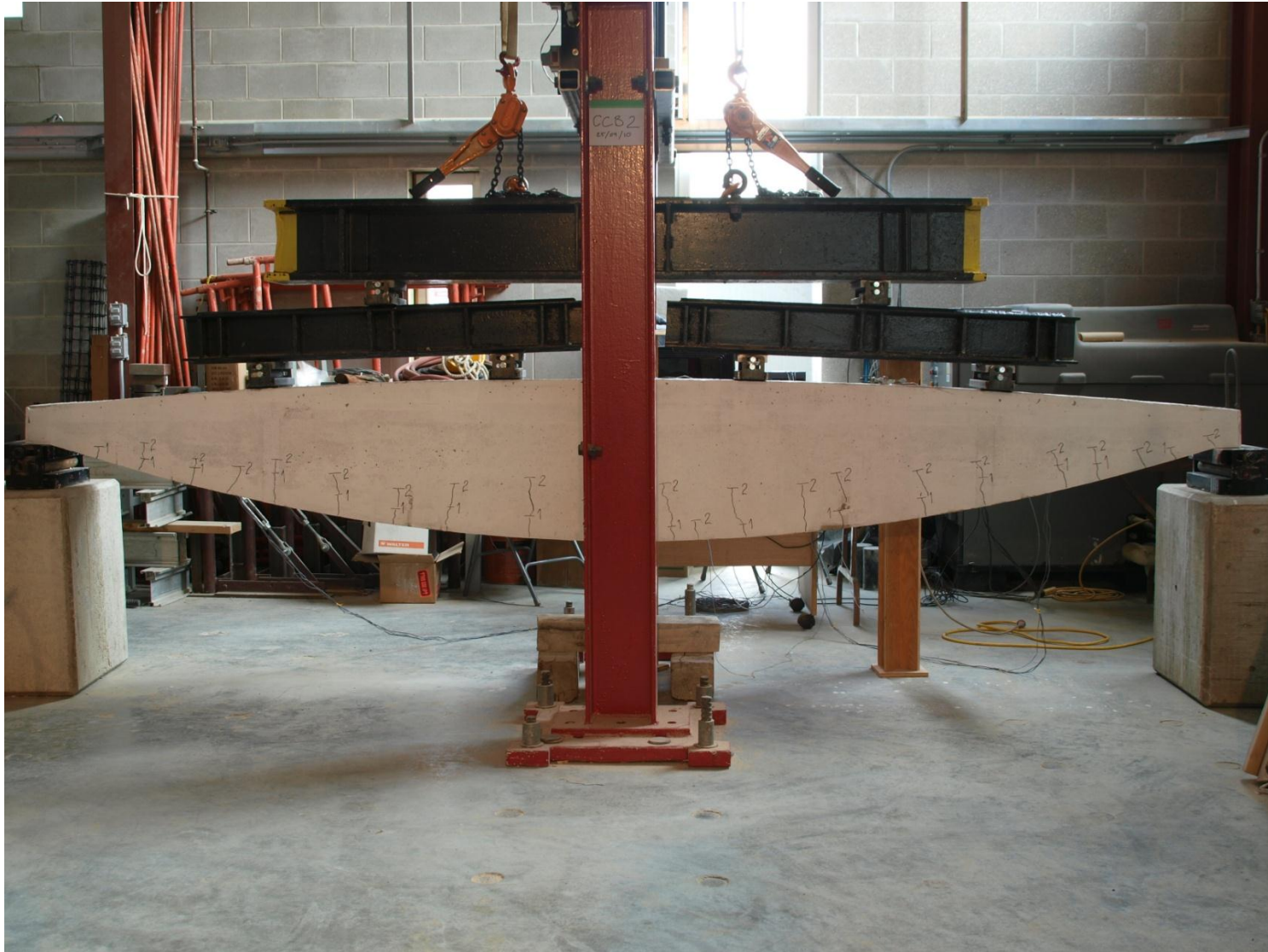
Figure 5.109 – CCB2 – Crack propagation at 60 kN
