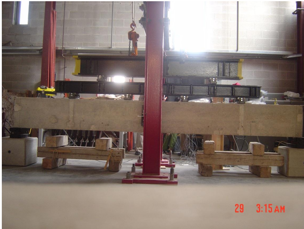
Figure 5.57 – Uniformly distributed crack propagation
