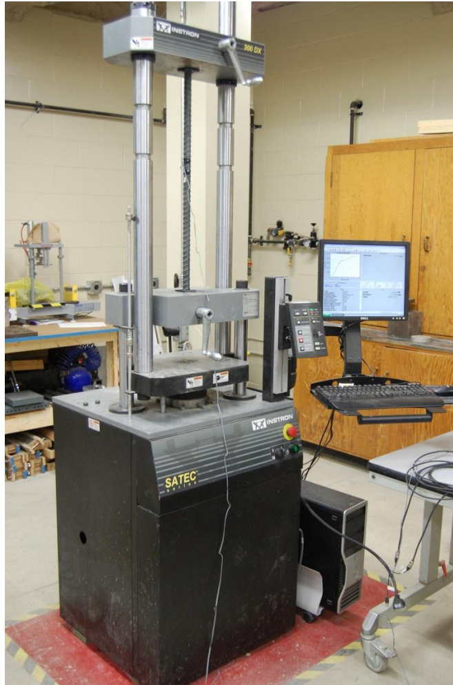
Figure 5.14 – Reinforcement tension test setup
