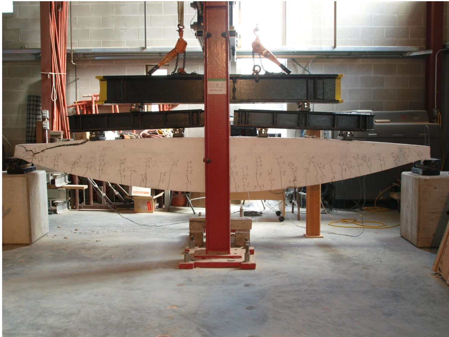
Figure 5.114 – CCB2 – after failure at 200 kN
