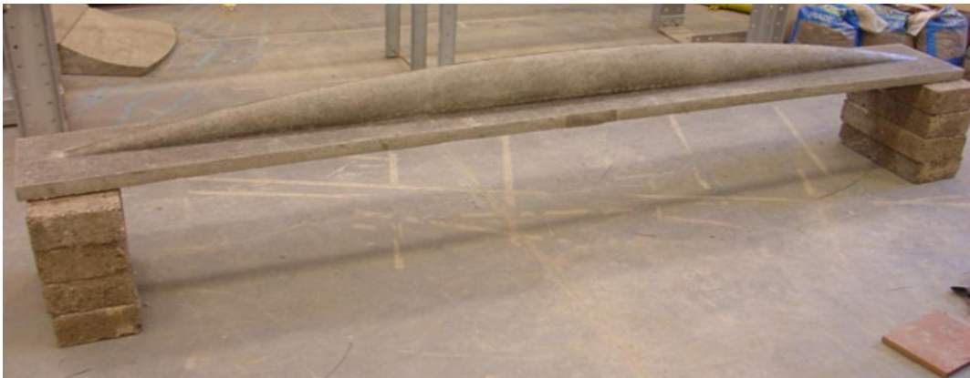
Figure 3.15 – Form-active beam (Lee/Pedreschi)
