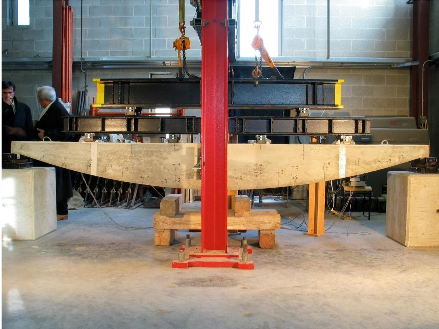
Figure 5.9 – Crack propagation at 45kN
