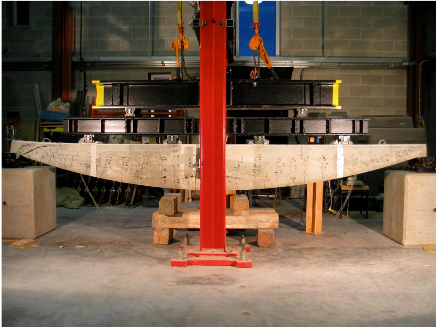
Figure 5.11 - CB3 After the failure
