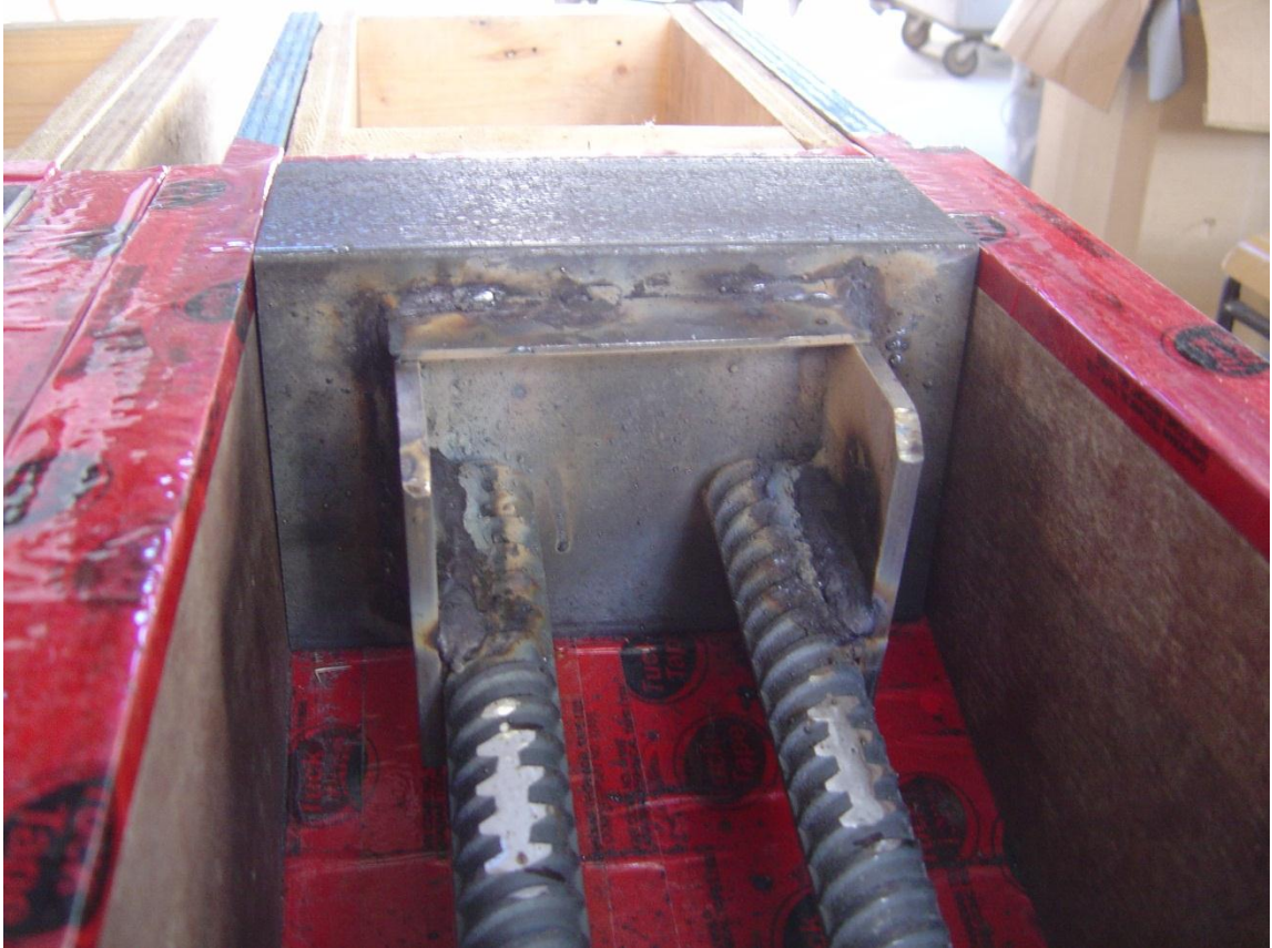
Figure 4.41 – End-angle configuration for ECB-RA1 and ECB-RA2.
