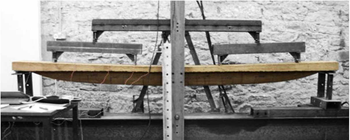
Figure 3.18 – Six-point loading (Lee/Pedreschi)
