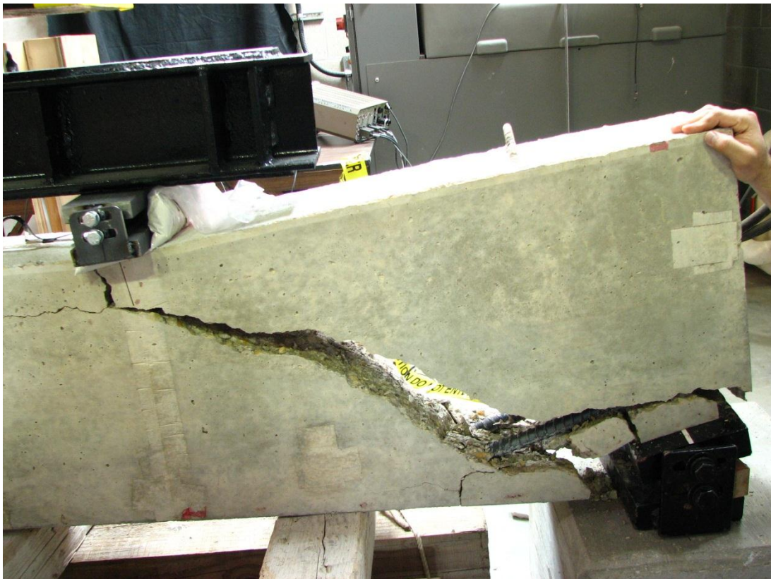
Figure 5.48 – Close-up of the failure end of RB1
