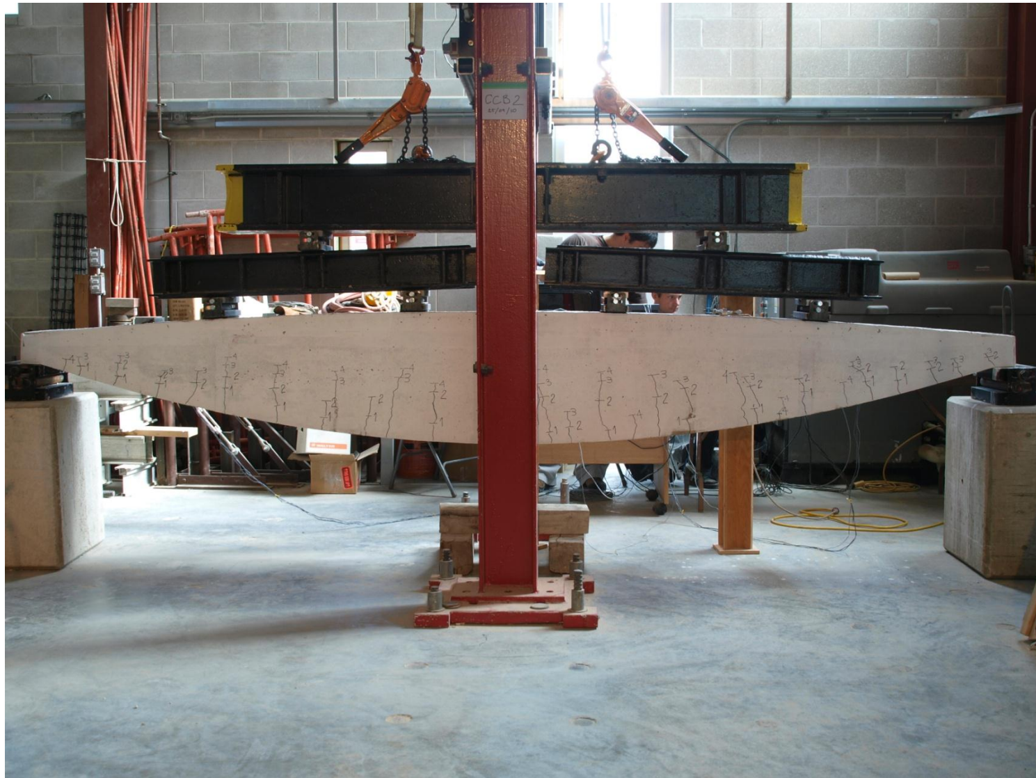
Figure 5.111 – CCB2 – Crack propagation at 100 kN
