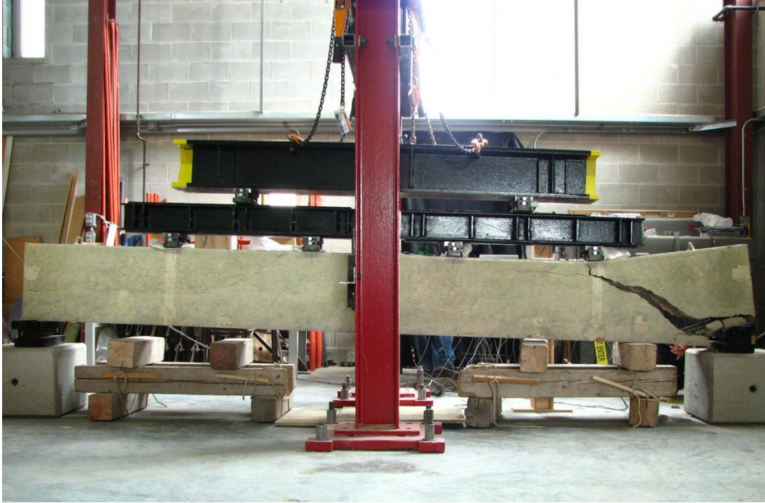
Figure 5.47 – RB1 at failure
