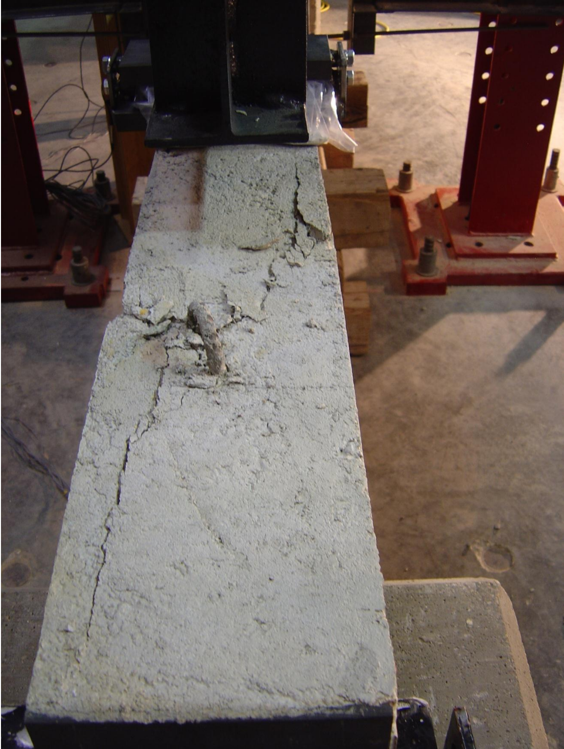
Figure 5.39 – The failure end at the top of the beam. Concrete is not crushed but slipped horizontally
