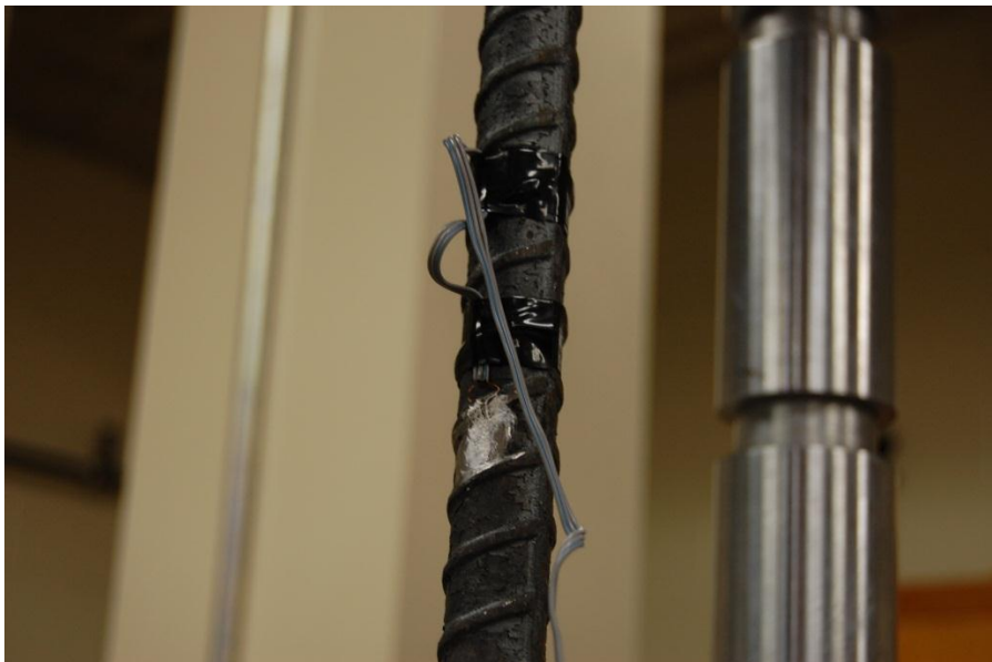
Figure 5.13 – Strain gauge on reinforcement for tension test
