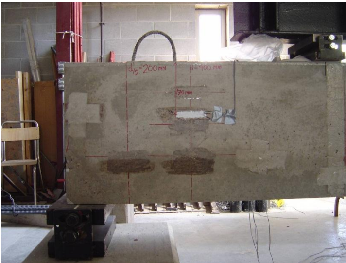
Figure B21 – Location of strain gauges on the side of the beam
