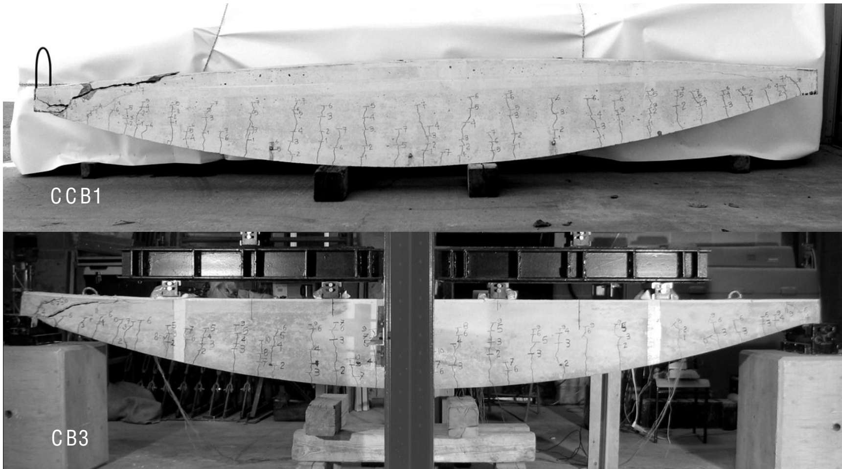
Figure 5.119 – Same failure mode and pattern for CCB1 (above) and CB3 (below)
