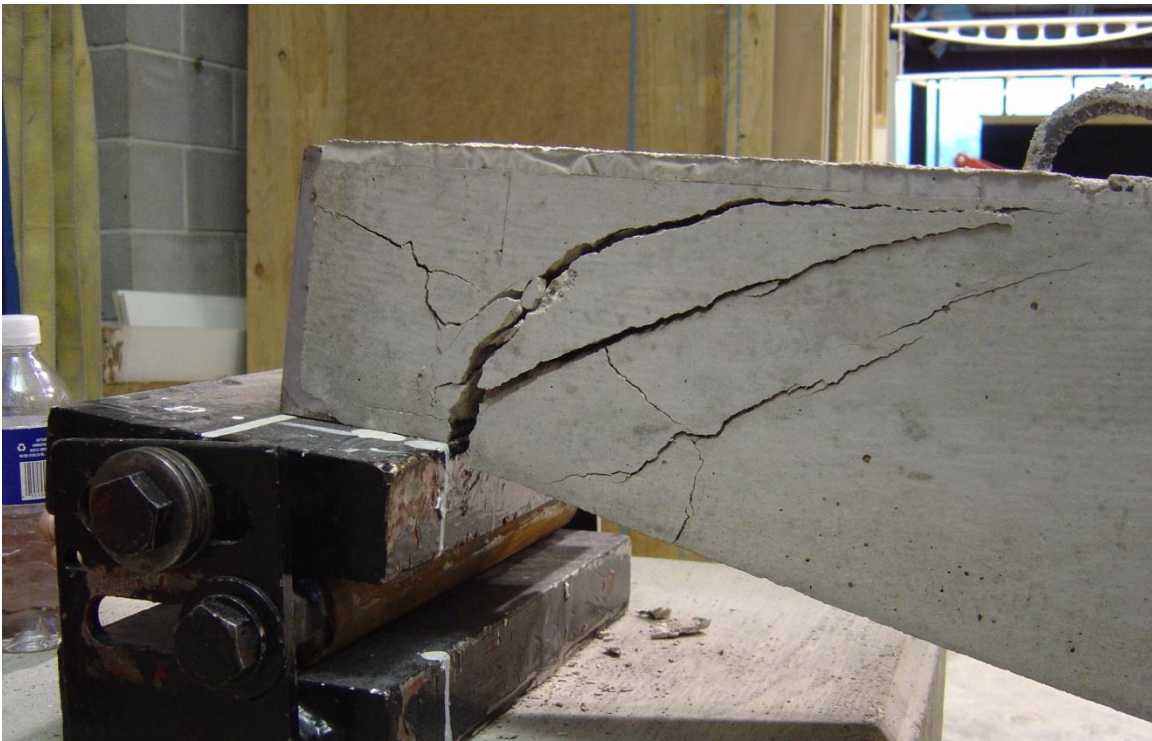
Figure 5.33 – Failure end detail for CB2
