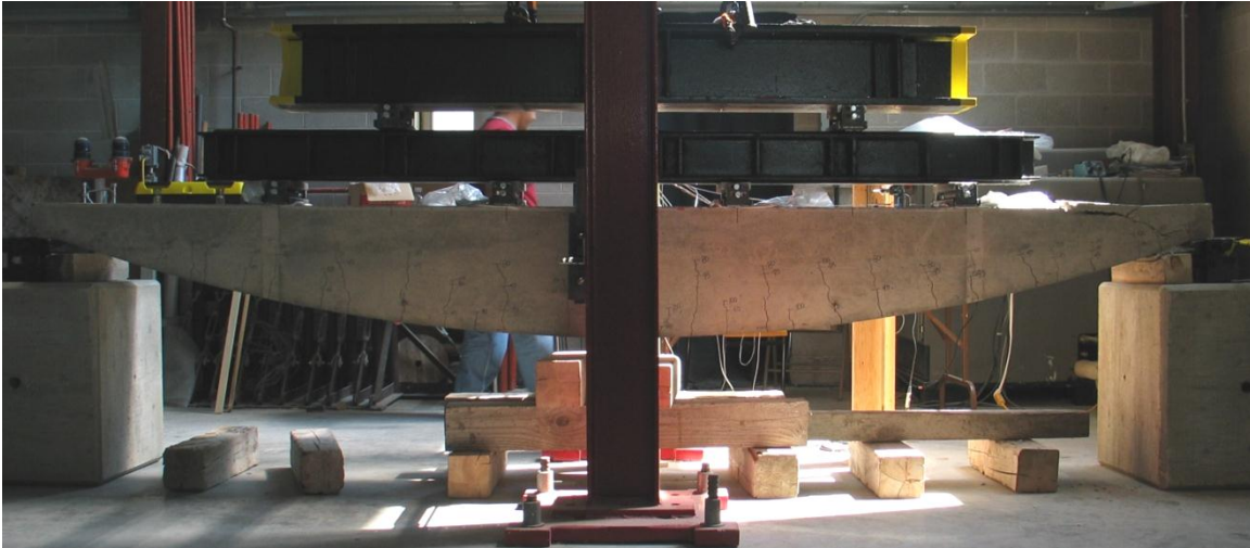
Figure 5.25 – Beam CB1 at final failure
