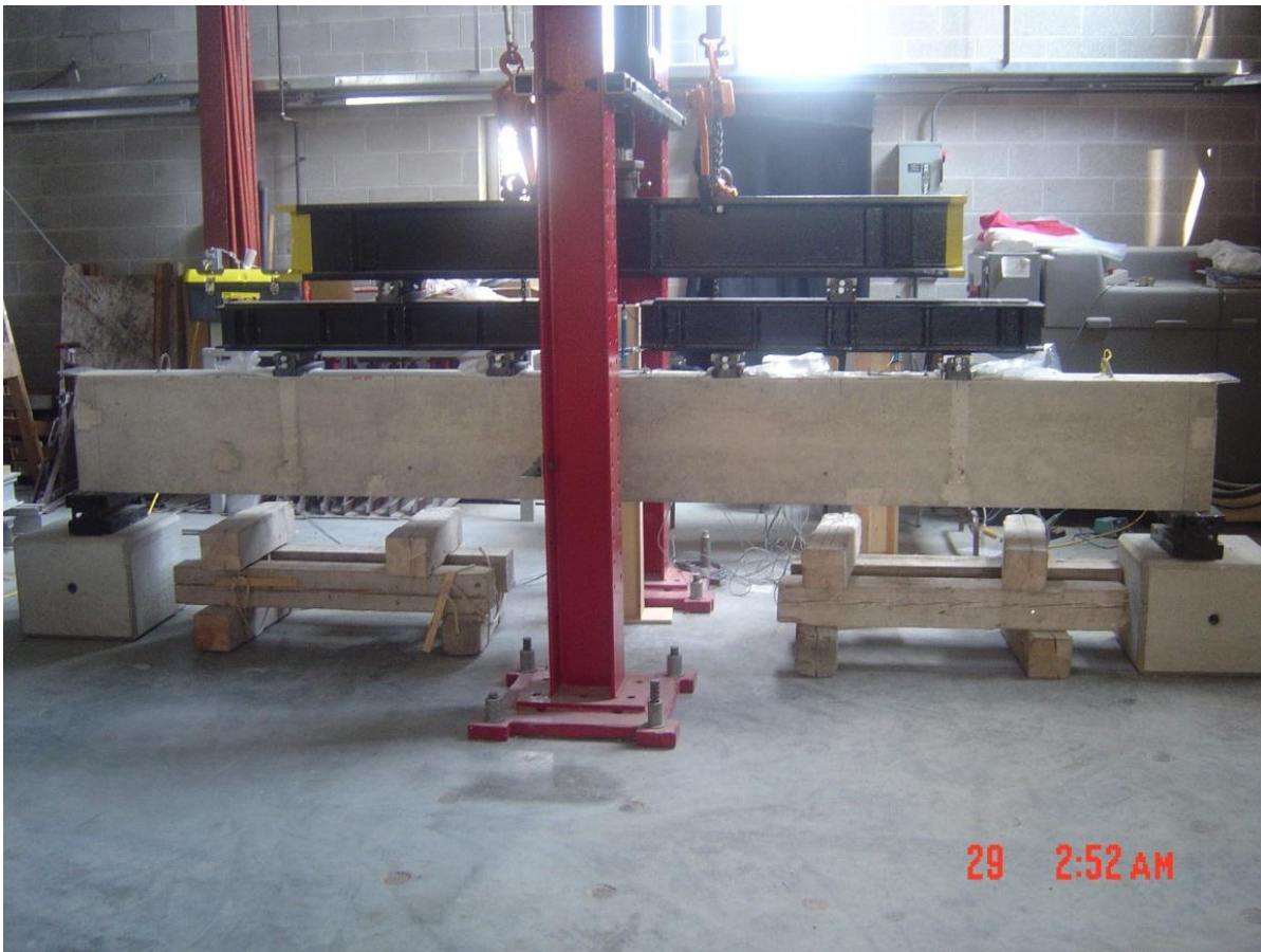
Figure 5.56 – Initial cracks not at centre-span
