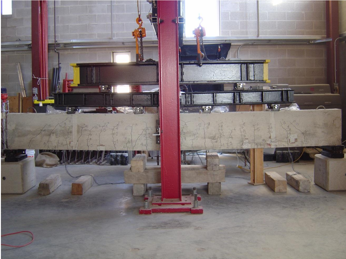
Figure 5.71 – RB3 (CSA designed beam) during testing
