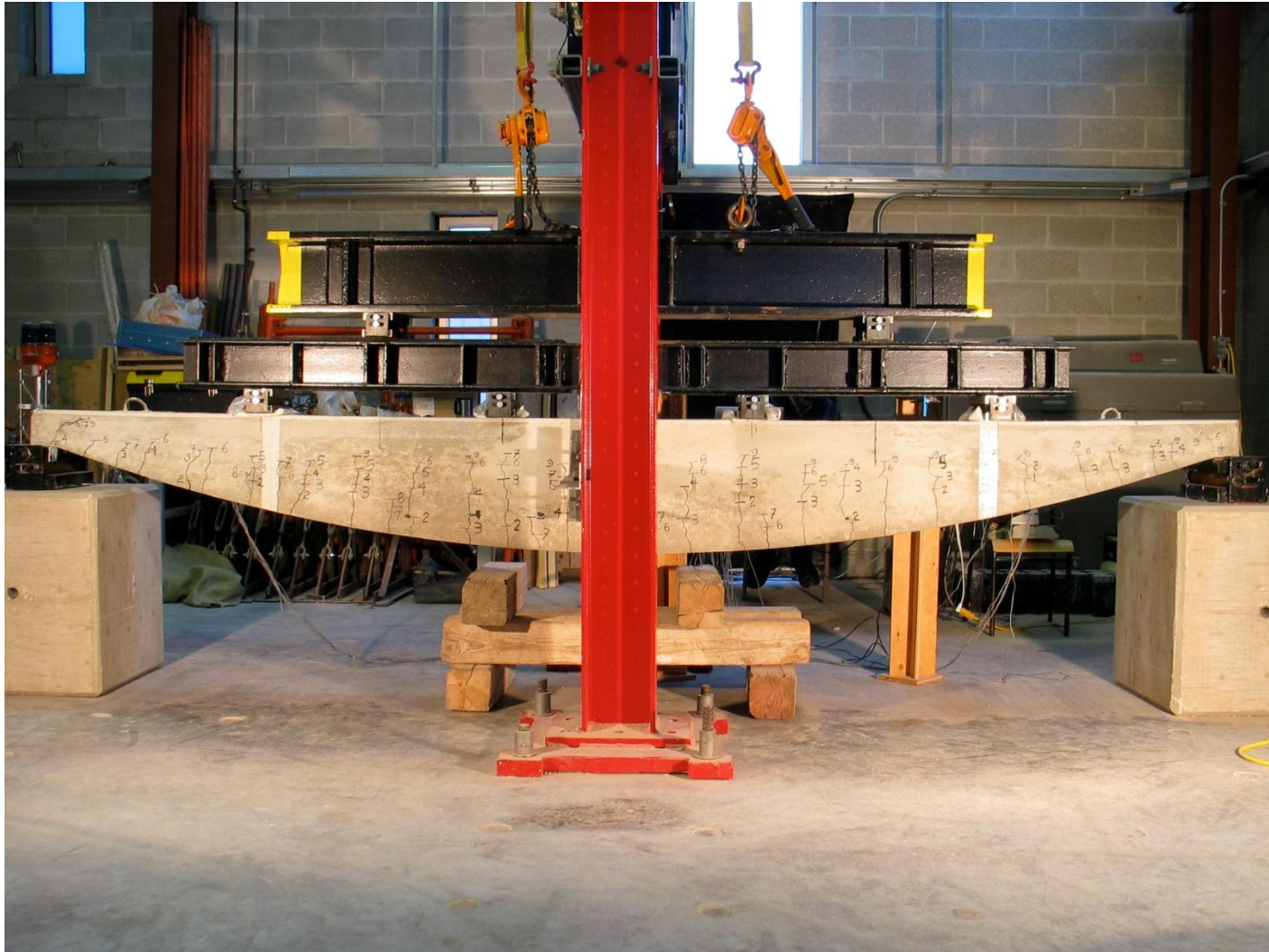
Figure 5.10 – Crack propagation at 140kN
