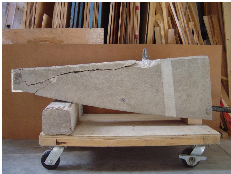
Figure 5.86 – ECB2 after testing. Crack pattern
