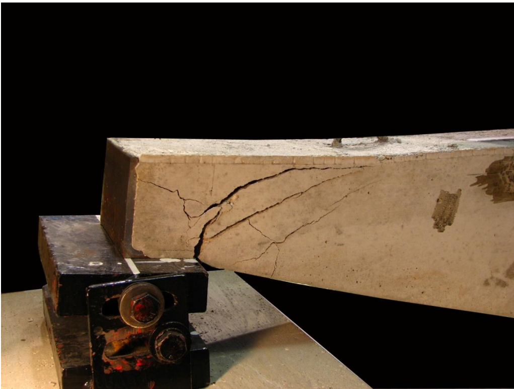
Figure 5.22 – CB2's end failure
