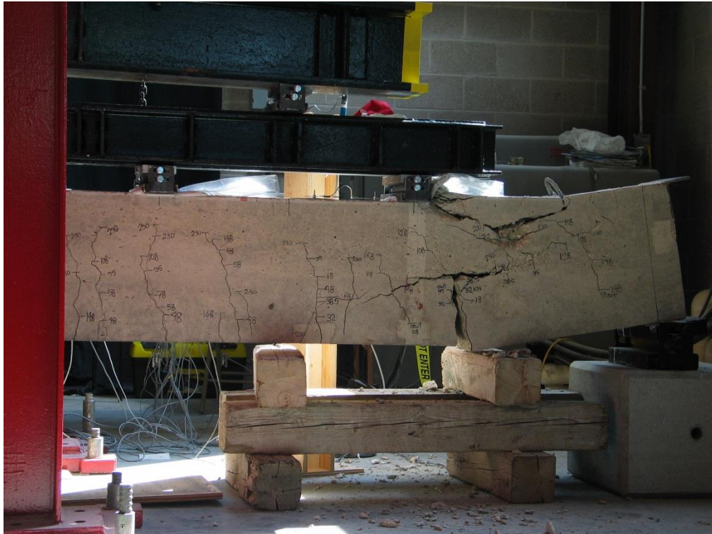
Figure 5.62 – Failure end of RB2
