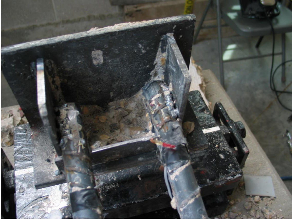
Figure 5.24 – Weld quality investigation, CB1
