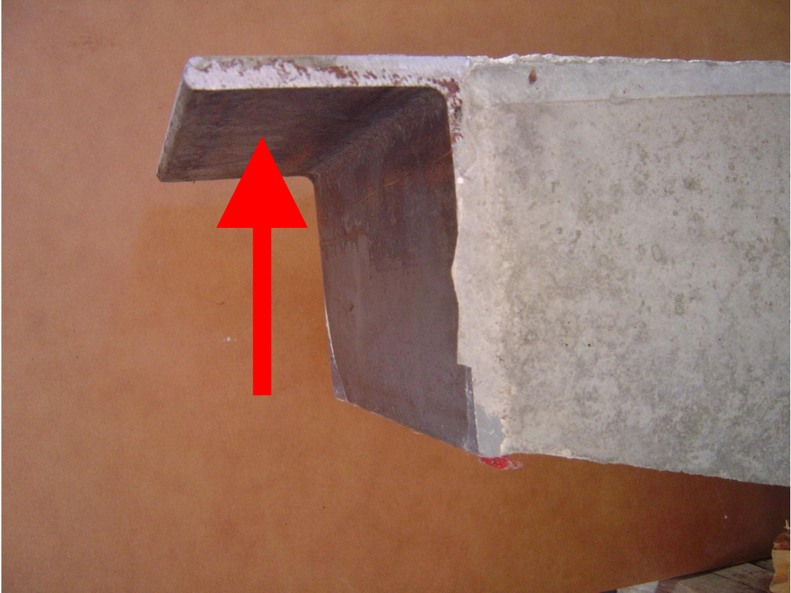
Figure 5.88 – Close up of the end angle, the arrow indicates the support point
