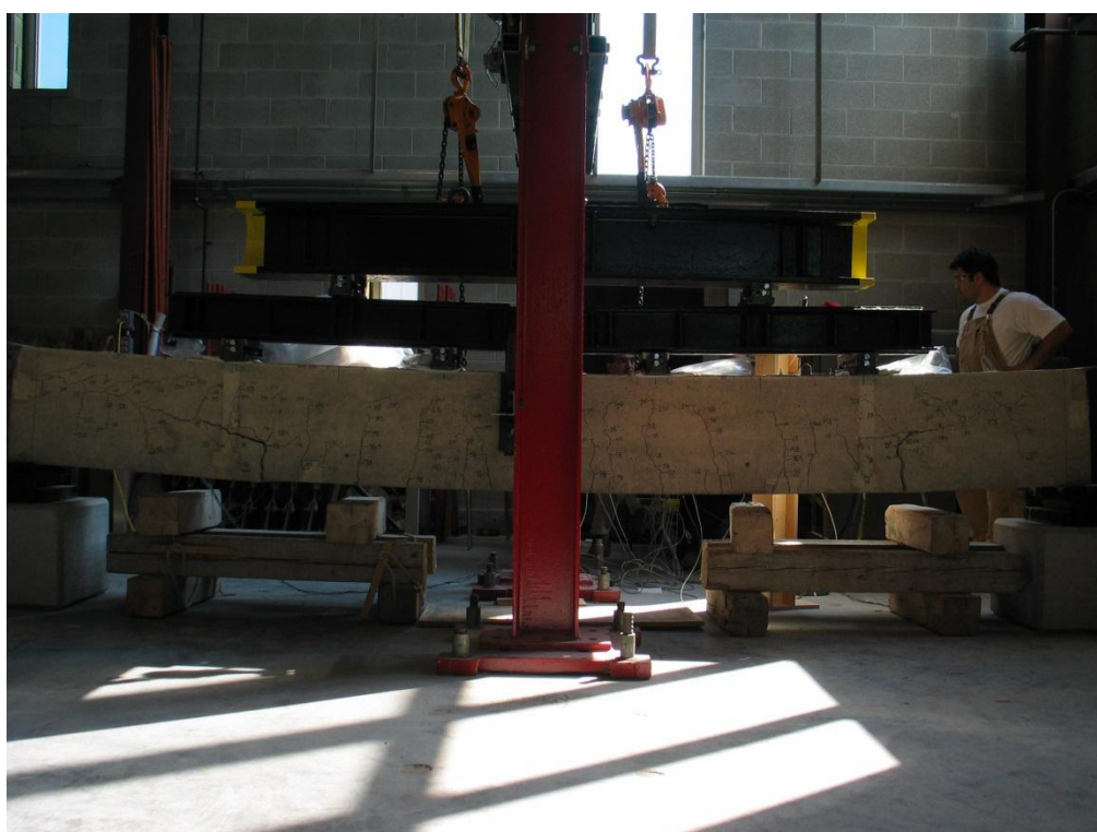
Figure 5.60 – RB2 prior to final failure
