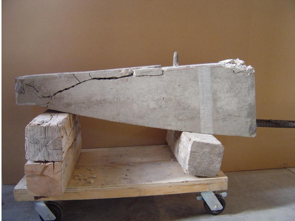
Figure 5.85 – ECB1 after testing. Crack pattern
