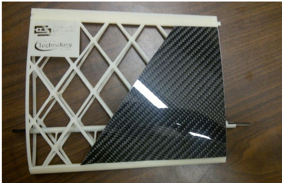
Figure 22. Prototype RP frame module with carbon fibre spar and veneer installed
