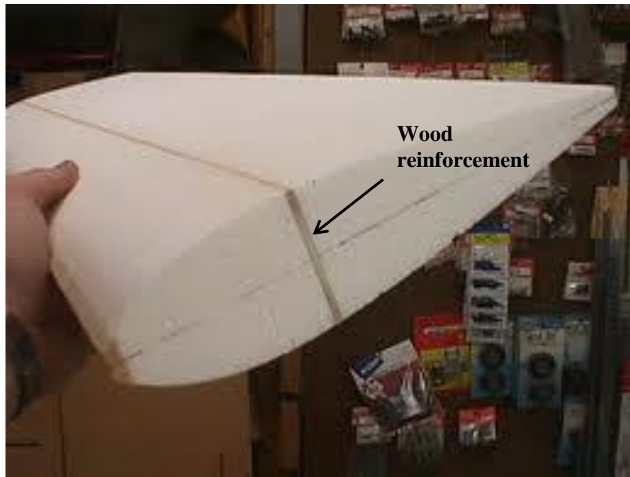
Figure 2. Foam wing shaped with hot wire cutter reinforced with wood [7]
