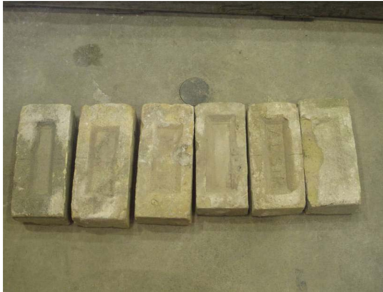
Figure 68: Oven dry brick specimens
