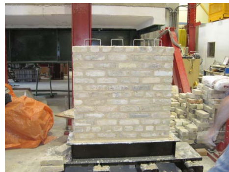
(f) Wall without concrete top beam
