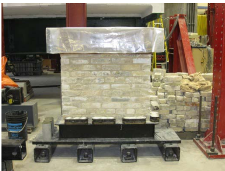
(g) Casting of concrete top beam
