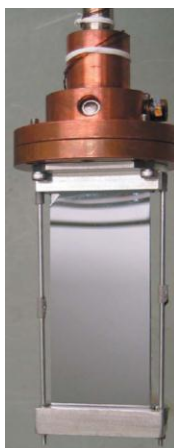
Figure 3.3. Photograph of the silicon flat plate sample holder that was used to obtain the neutron diffraction patterns of GdGa (Ryan & Cranswick 2008).
