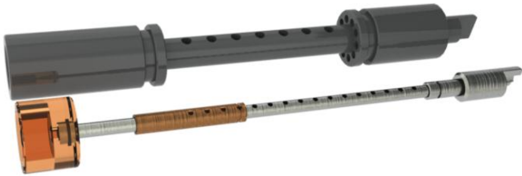
Figure 4.17 Scaffold holder designed for microvessels.
