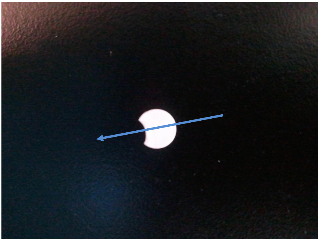
Figure 3.4 Partially punched membrane disk for indication of alignment direction.
