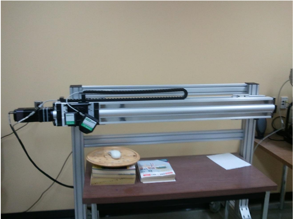
Figure 3.12 The 3D laser scanner.
