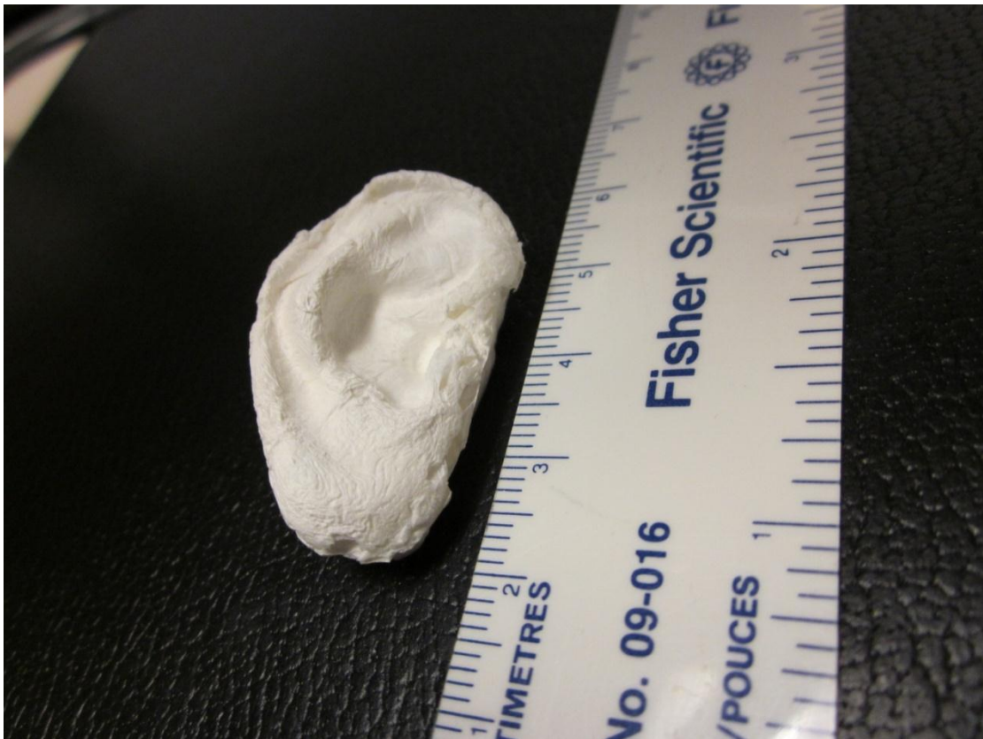
Figure 4.15 Human ear shaped nanofibrous scaffold.
