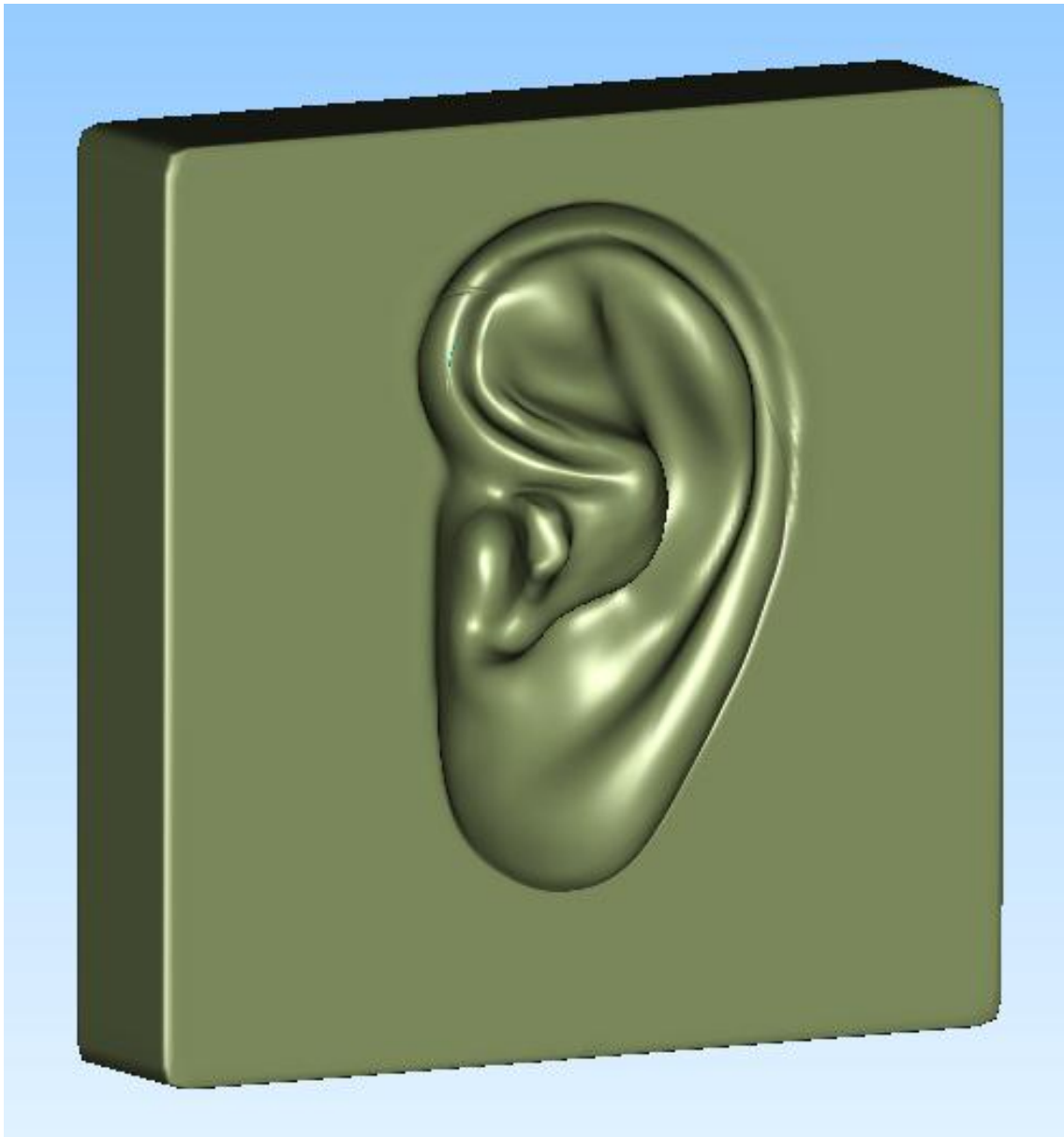
Figure 3.17 The final negative mold after subtraction.
