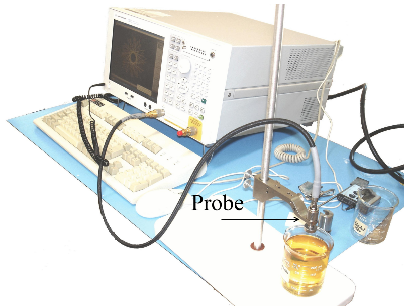
Figure A.1: Agilent 85070E dielectric measurement probe connected to VNA.
