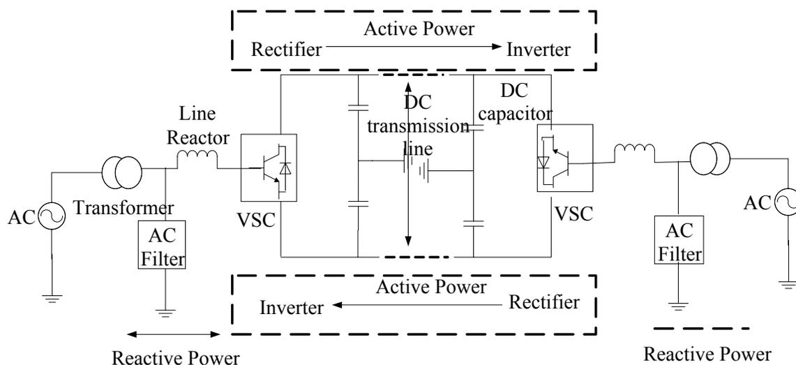
Figure 2-1: Topology of a VSC-HVDC system
