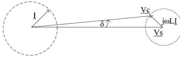
Figure 2-12: Phasor representation of model 2.8
