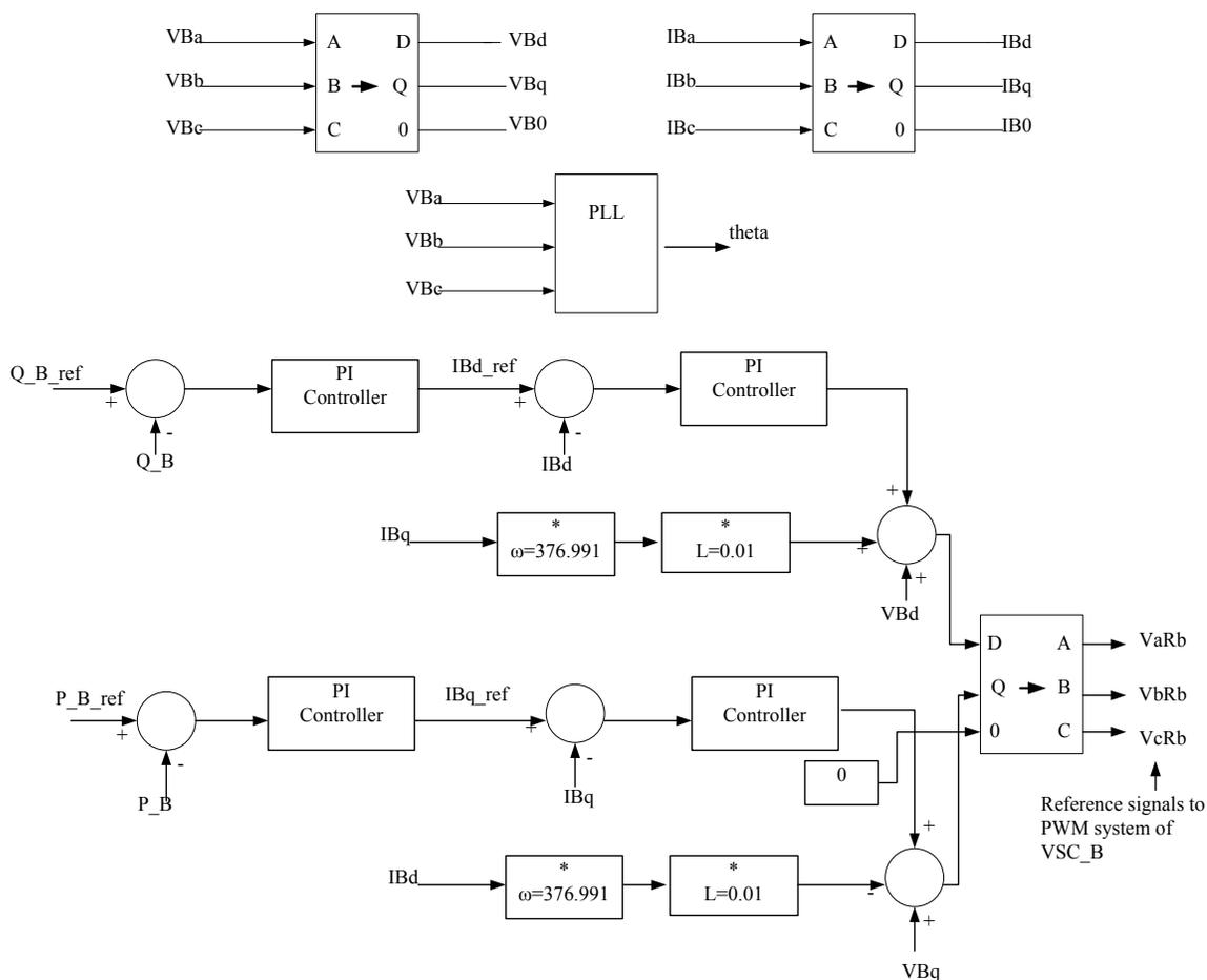
Figure 3-3: Control System VSC-B
