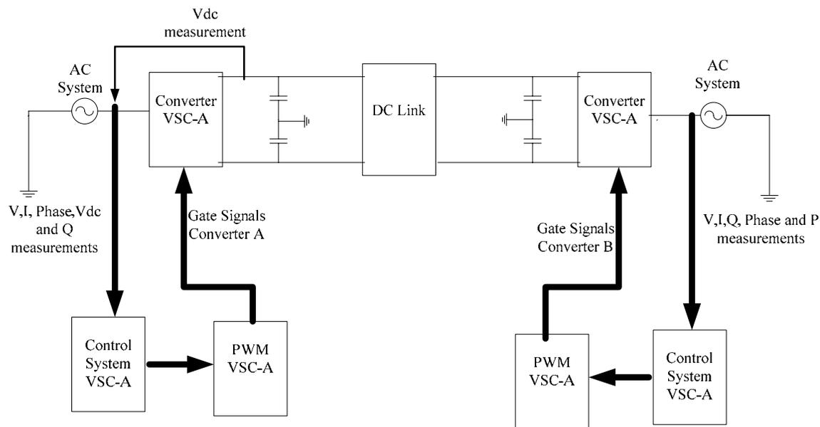
Figure 3-8 : Complete system in block diagram form
