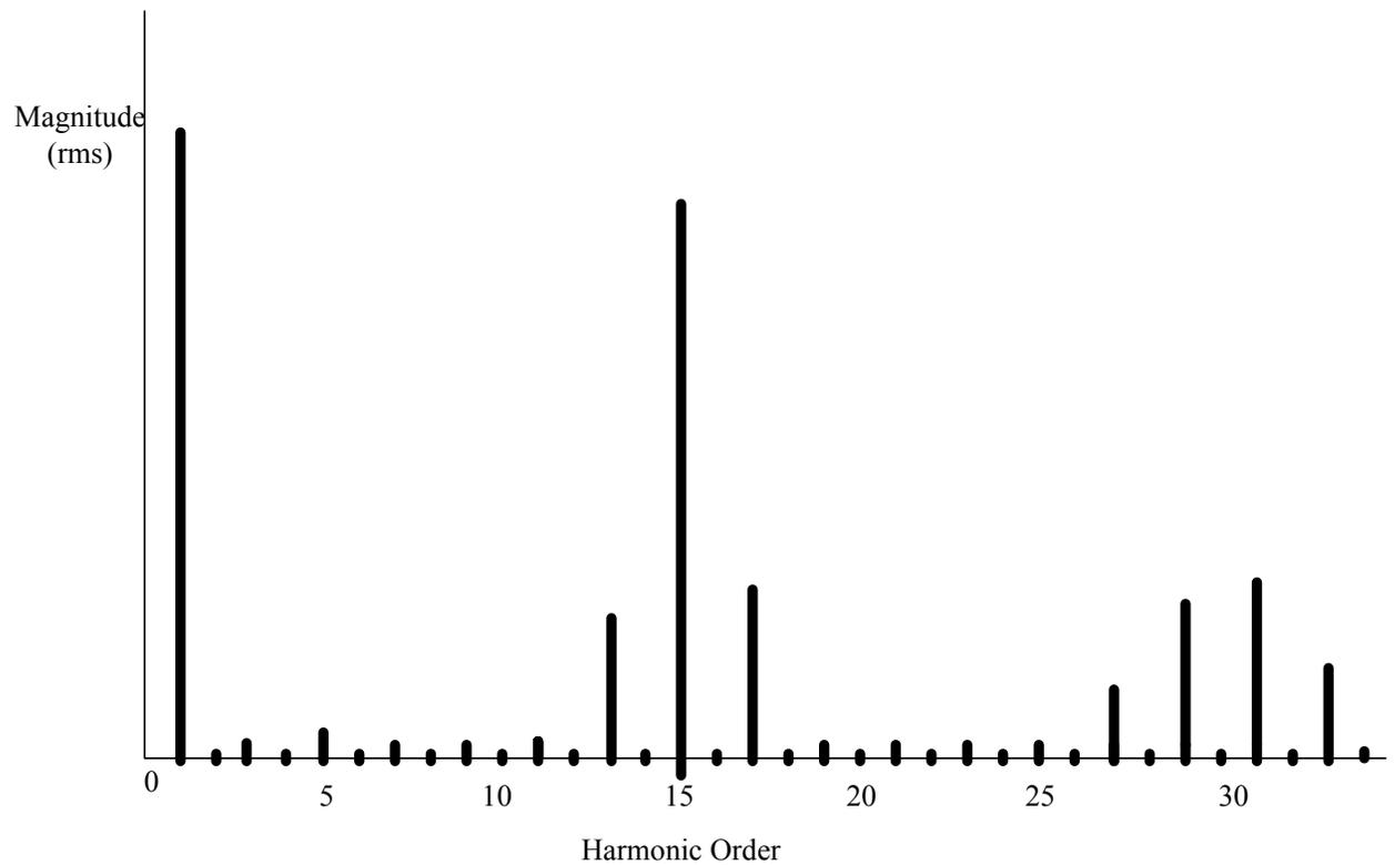
Figure 2-9 : Harmonic Spectrum when frequency ratio is 15
