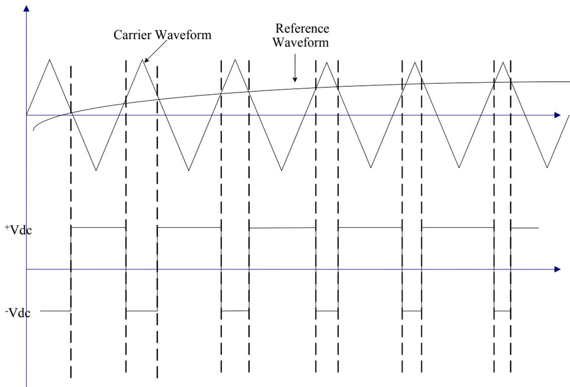
Figure 2-6: Waveforms for PWM general case
