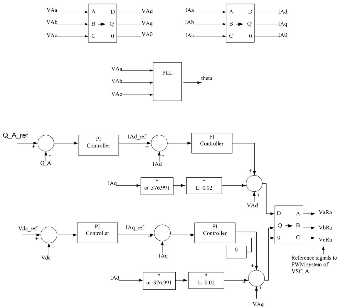
Figure 3-2: Control System VSC-A
