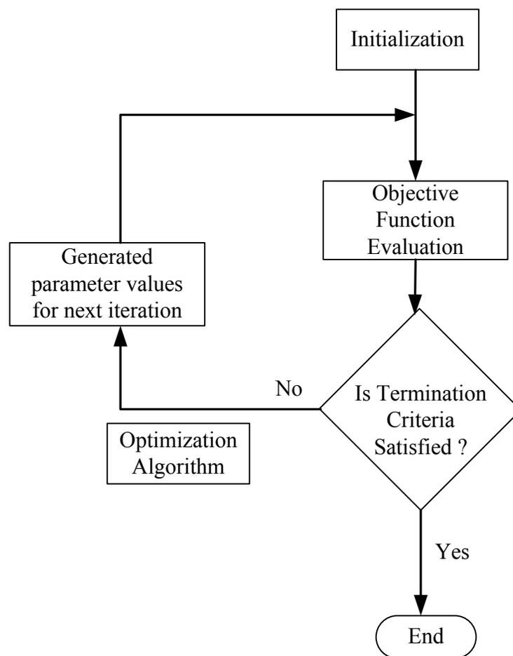
Figure 3-5 : Basic Interface between optimization and transient simulation [3]
