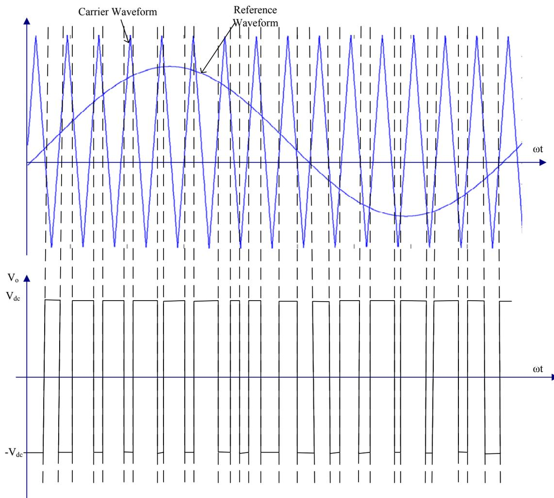
Figure 2-8: Waveforms for sinusoidal PWM
