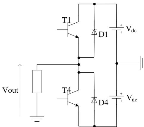
Figure 2-3 : Single leg of the Converter Bridge
