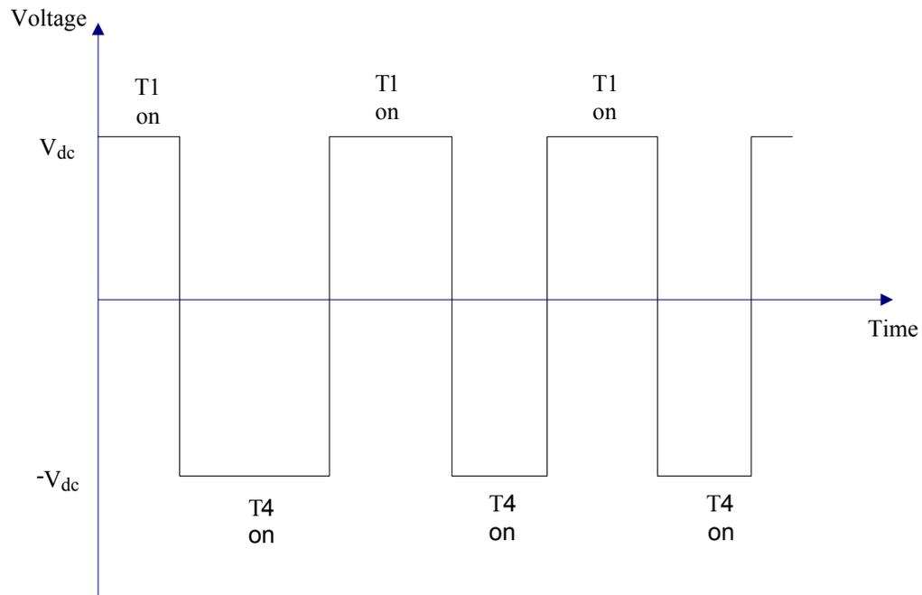
Figure 2-4 : Load voltage for a single leg
