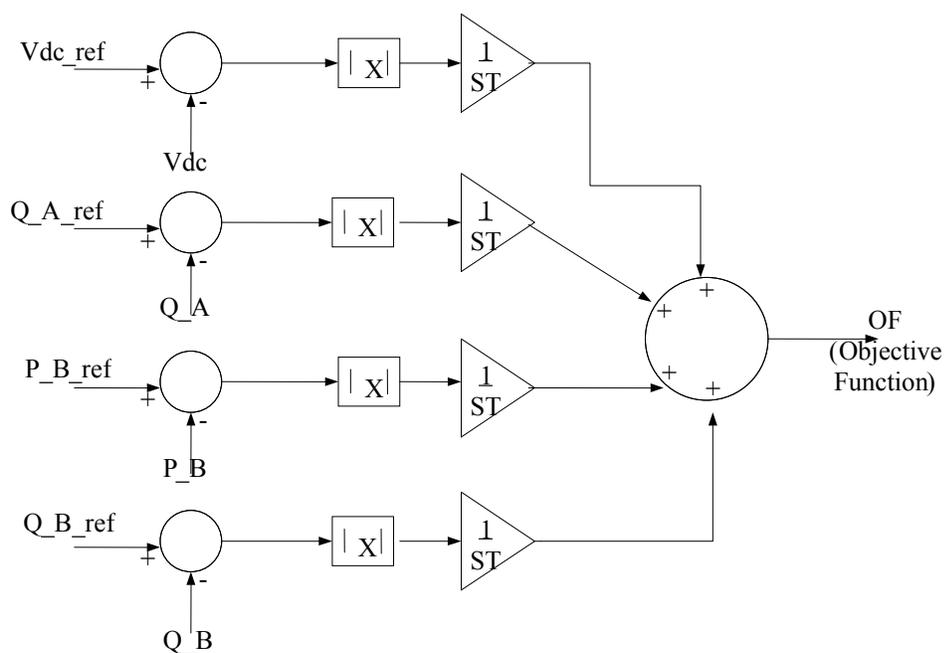
Figure 3-6 : Implementation of the objective function
