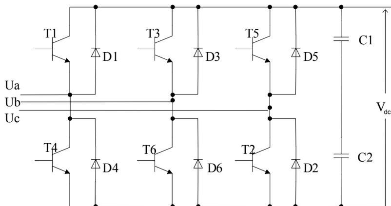
Figure 2-2: Two level VSC Converter Bridge
