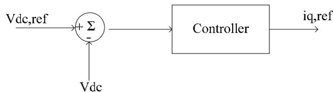
Figure 2-15: DC Voltage controller
