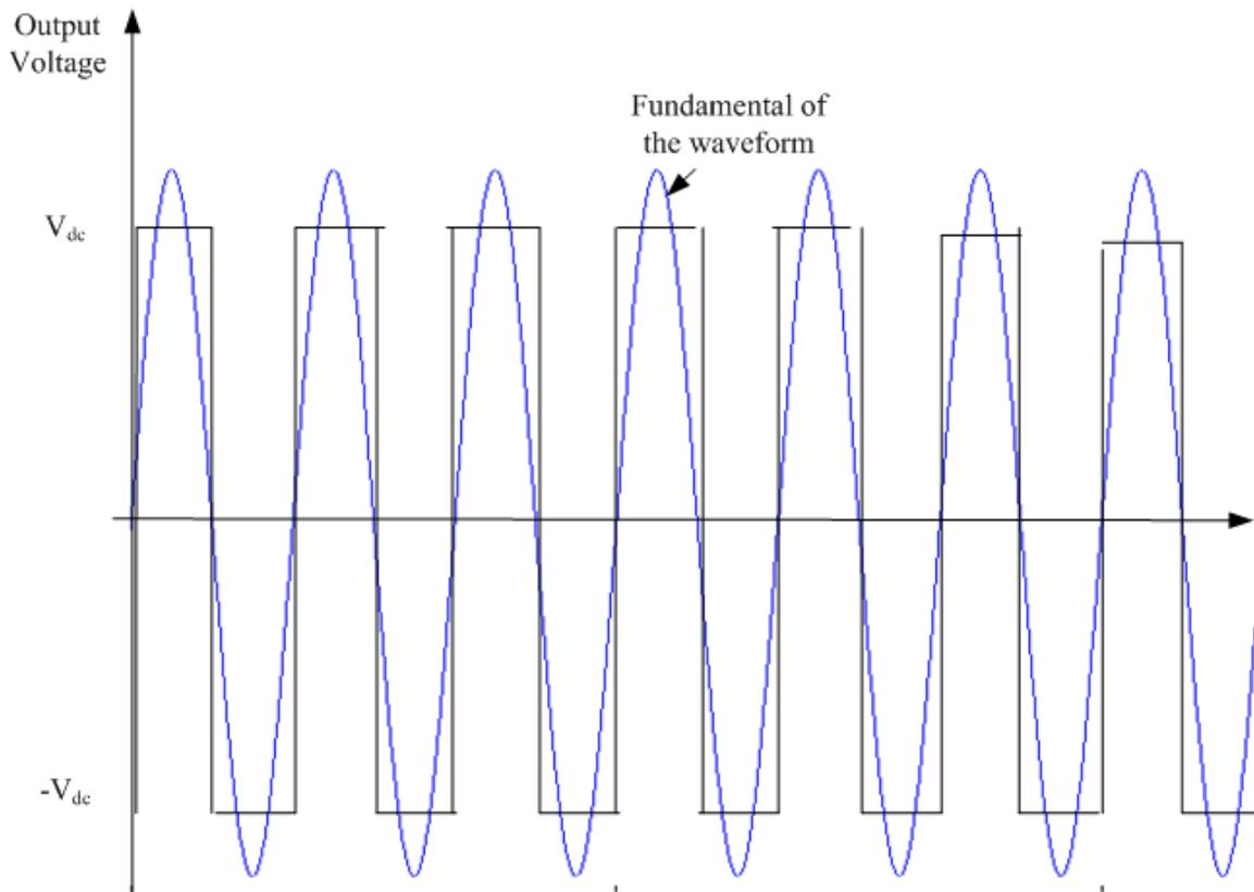
Figure 2-5 : Output voltage and the fundamental of it under square wave operation
