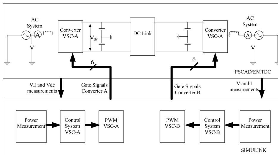
Figure 4-3: Interaction between PSCAD and SIMULINK
