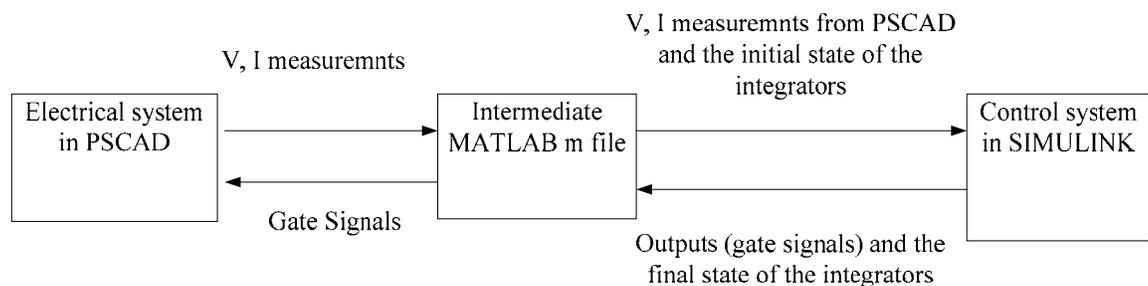
Figure 4-2 : Communication between PSCAD and MATLAB/SIMULINK
