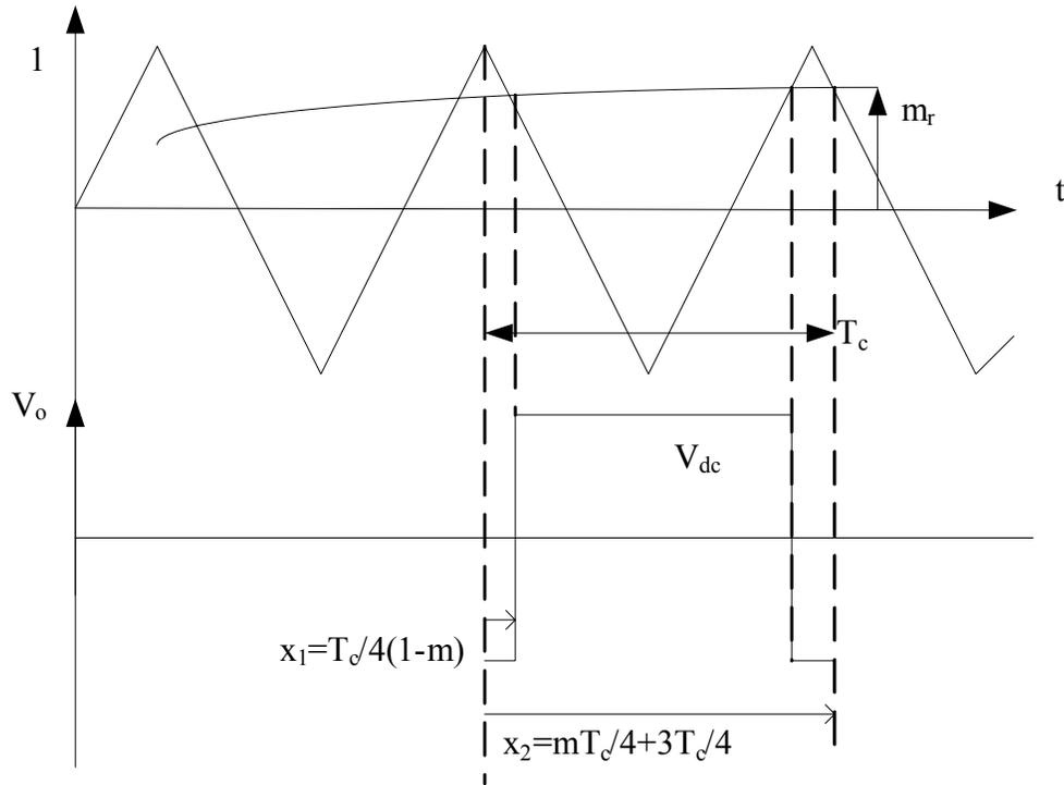
Figure 2-7 : Development of Modulation Index
