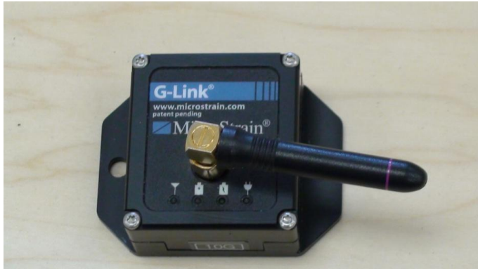
Figure 3a. The wireless tri-axial accelerometer used in the study is shown.
