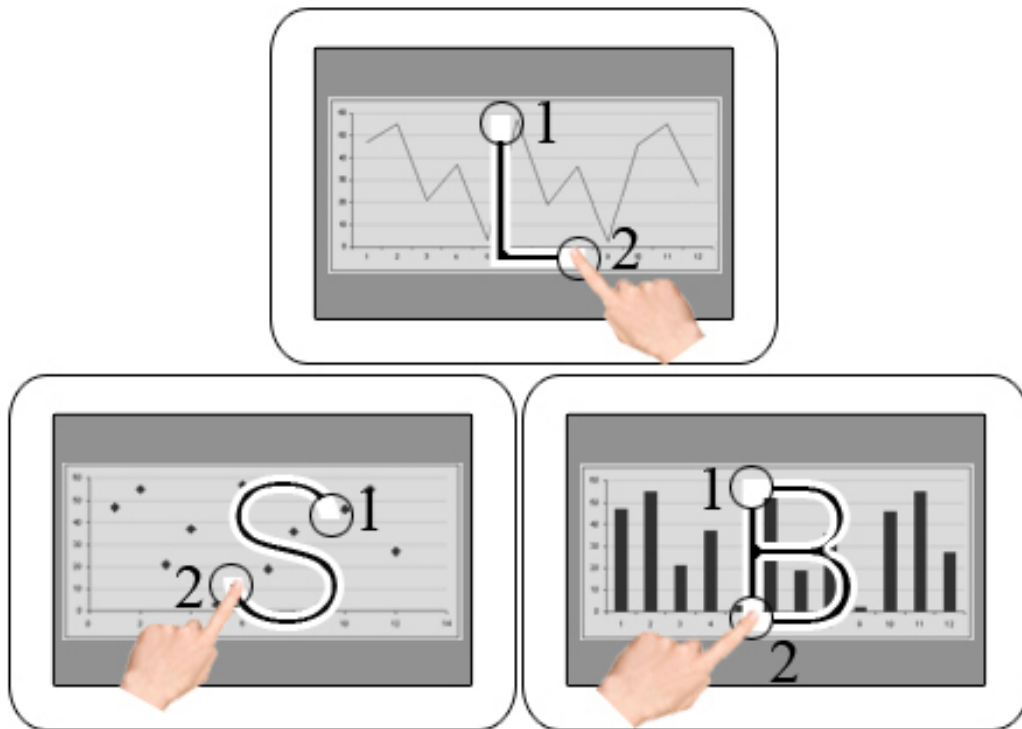
Figure 31: The interface provides the user with ability to choose different chart types (line, scatter or bar) for representing a graph. The user makes a finger gesture from the starting point (1) to the ending point (2) to invoke the change.
