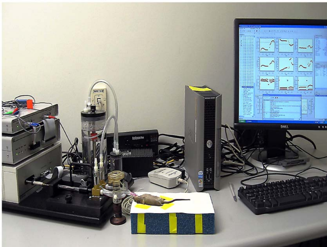
Figure 6: Tracheotomy and lung function analysis using the flexiVent ventilator. Pictures showing a mouse with a (A) tracheotomy and (B) lung function testing using a flexiVent ventilator.
