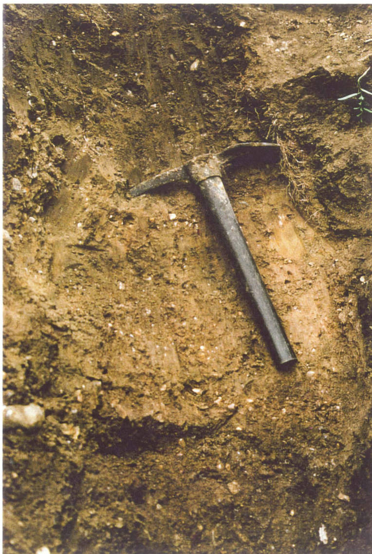
Fig. 3-1 A photograph of diamicton lithofacies (Dh) from a river-cut near the town of Wawanesa at Sec.23 Tp7 R17W (see also Fig. 3-18). The pick is placed over a pinkish olive till bed that is sandwiched by olive grey till beds above and below the pick. The pick handle is about 0.55 m long.
