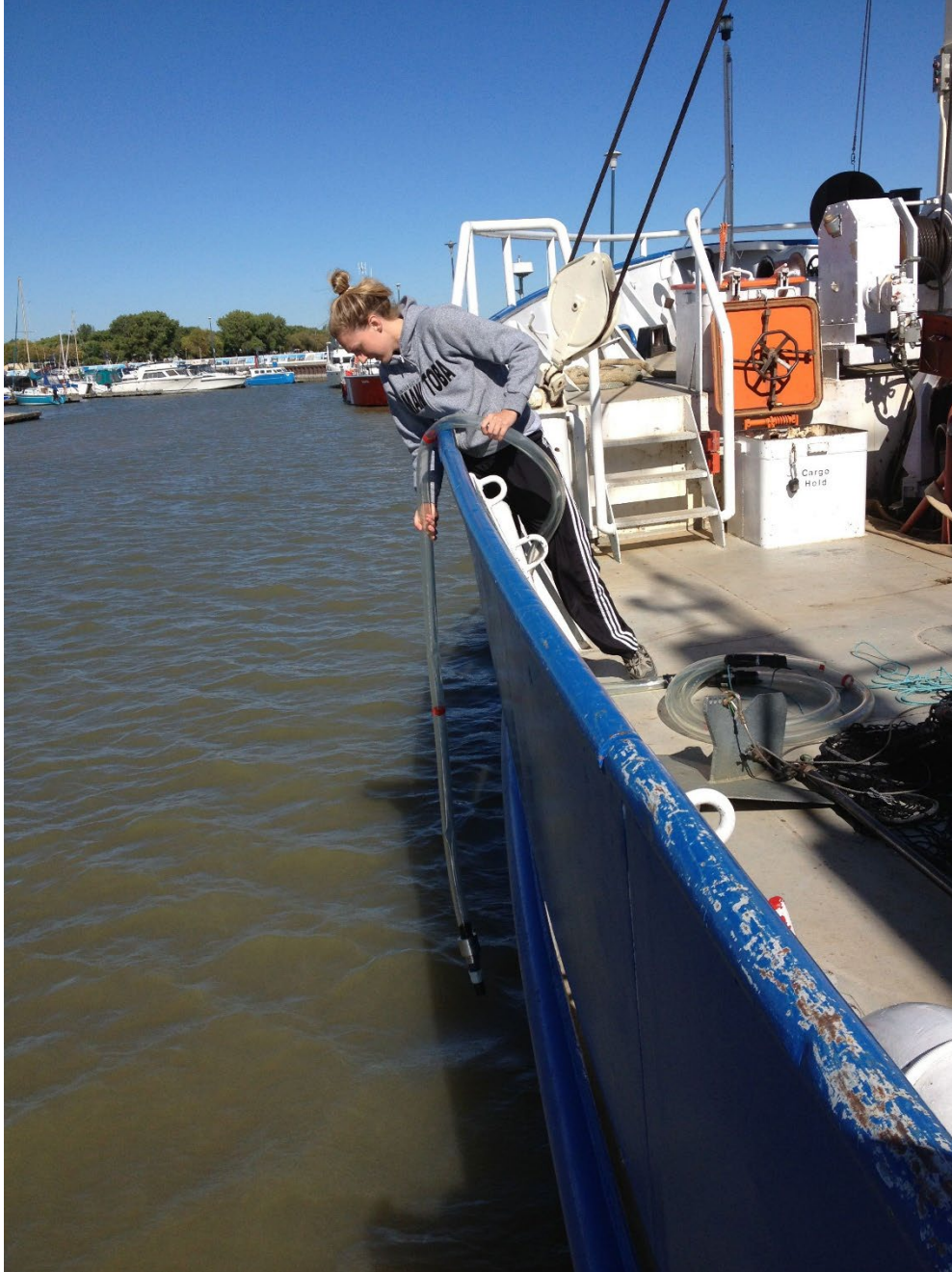
Figure 8. Picture of integrated tube sampler in use off the front deck of the MV Namao . The integrated tube sampler is used at all 14 W stations on Lake Winnipeg to get a euphotic sample. The euphotic depth is measured as the depth in the water column where 1% of light penetrates (photo taken by Marianne Geisler).
