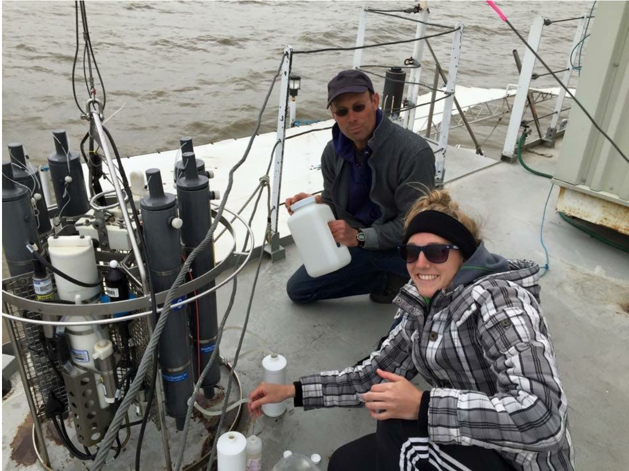
Figure 13. Desiree Stratton filling sampling bottles from Environment and Climate Change Canada's Seabird Rosette off the top deck of the MV Namao on Lake Winnipeg. The Seabird Rosette can take water samples at any depth in the water column as well as in situ data such as temperature, conductivity, DO, turbidity, chlorophyll a and photosynthetically active radiation (PAR) (photo taken by Tracie Greenberg).
