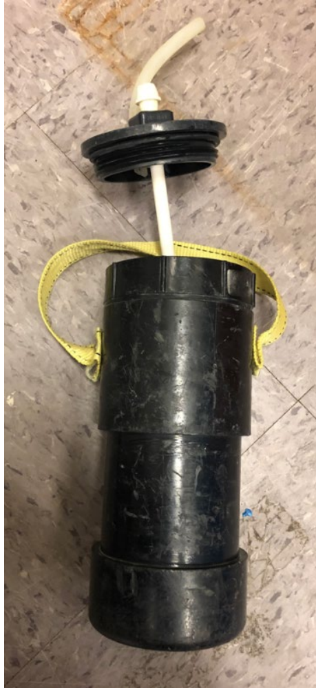
Figure 9. Picture of a DO sampler. The DO sampler is lowered down within the euphotic zone off the front deck of the MV Namao and used at all 14 W stations. The euphotic depth is measured as the depth in the water column where 1% of light penetrates (photo taken by Desiree Stratton).
