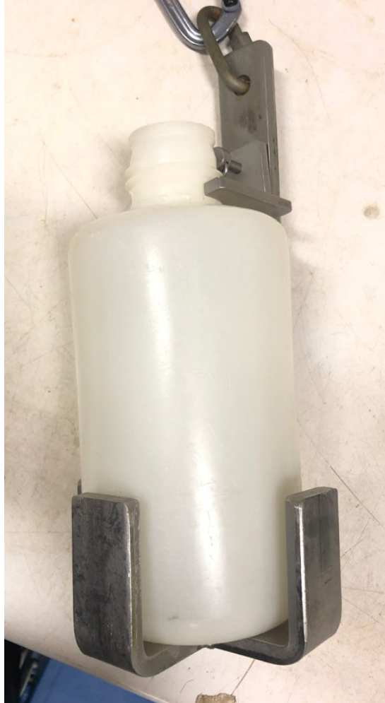
Figure 10. Picture of a weighted sampler. The weighted sampler was used at one-off algal bloom sites sampled off the MV Namao on the front deck. The weighted sampler was lowered down from 0-0.5m below the surface and filled (photo taken by Desiree Stratton).
