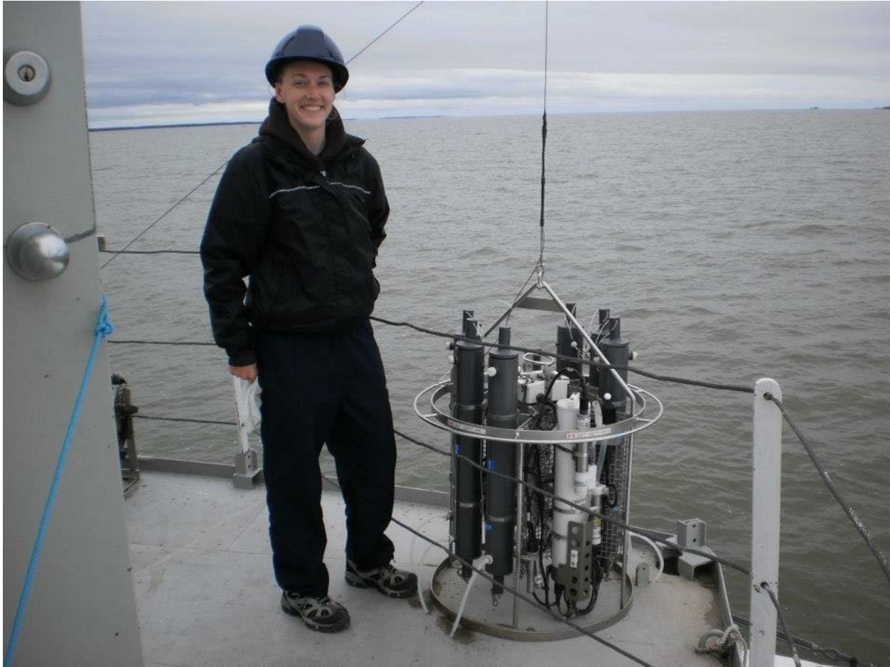
Figure 12. Desiree Stratton next to Environment and Climate Change Canada's Seabird Rosette on the top deck of the MV Namao on Lake Winnipeg. The Seabird Rosette can take water samples at any depth in the water column as well as in situ data such as temperature, conductivity, DO, turbidity, chlorophyll a and photosynthetically active radiation (PAR) (photo taken by Tracie Greenberg).
