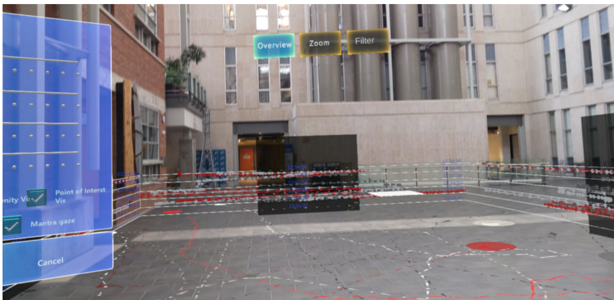
Figure 50: The implementation of the 'Overview first' step into SSMA visualization. At the top, the floating AR buttons Overview, Zoom, and Filter. The user can activate overview first step by pointing and pinching the Overview button.
