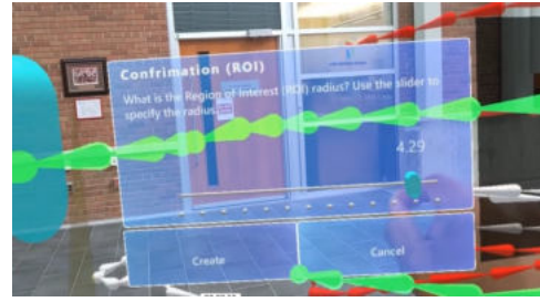
(b) Then, the user adjusts the cylinder's radius using a slider to select the desired area of interest.
