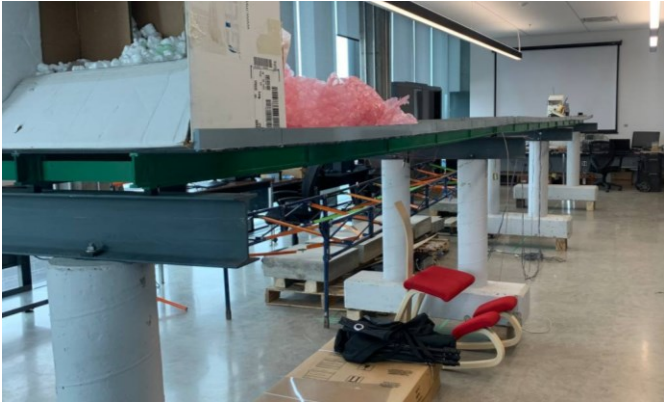
Fig 4.2. South Perimeter bridge small-scale model in the SHM laboratory
