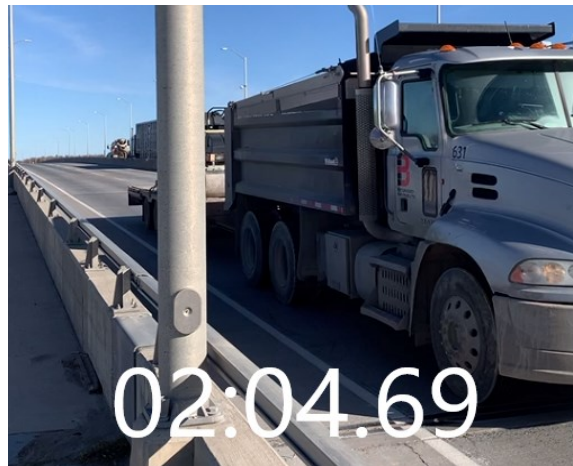
Fig 3.19. The entering time when the truck's front axle entered the span through the first expansion joint
