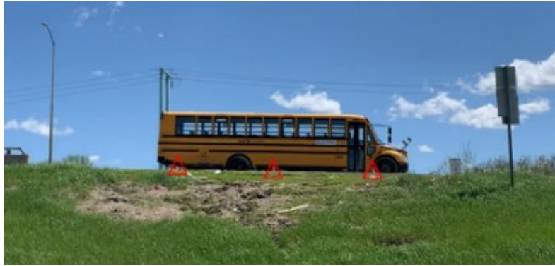
Fig 3.31. An example of a video frame with cones as a known-length scale.
