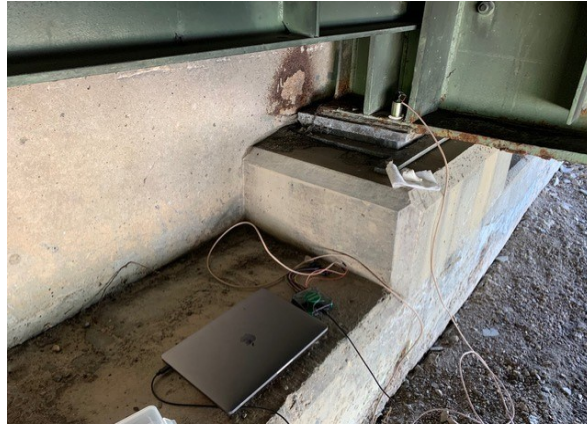
Fig 3.24. The geophone was attached with the twisted cable to the laptop through the Analog
