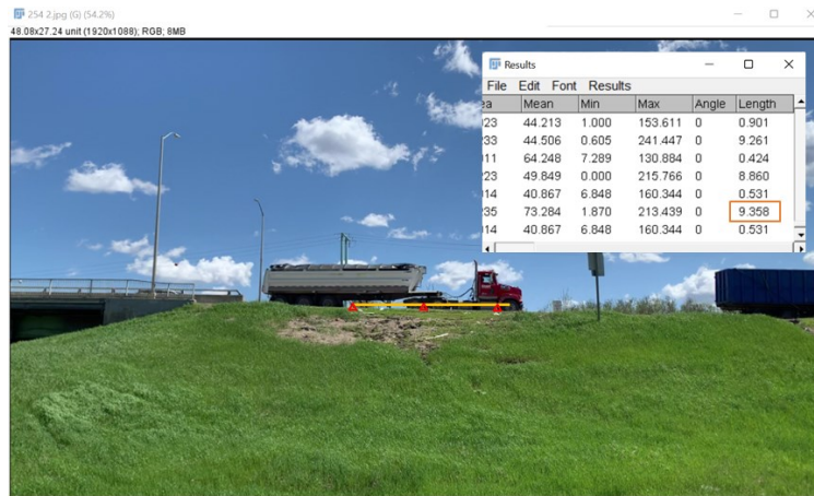
Fig 3.46. Displays the measured distance from the first wheel to the first pylon cone that was calculated as X1 through ImageJ software
