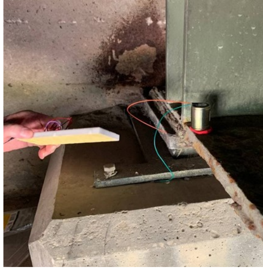
Fig 3.8. The geophone was attached to the teensy board with Arduino
