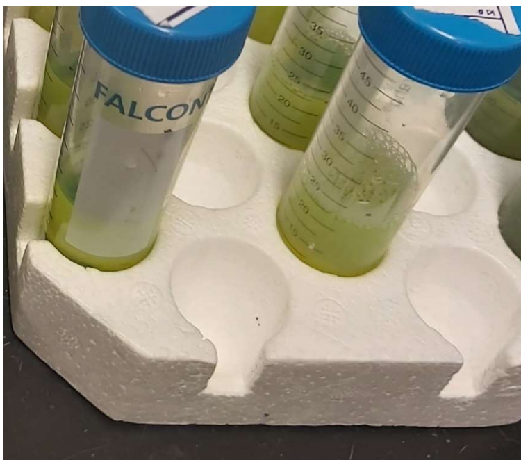
Figure 2- Samples prepared for Fluorescein Diacetate Assay test
