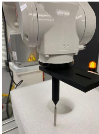
Figure 3.9: Robot tool calibration (TCP offset calculation)
