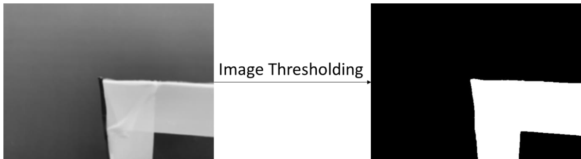
Figure 3.19: Image thresholding for corner detection
