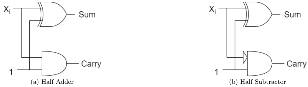
Figure 5.4: 1-bit Increment and Decrement using Half-adder or subtractor where the x_i is the input Bit and the Carry bit is propagated into the next bit's operation
