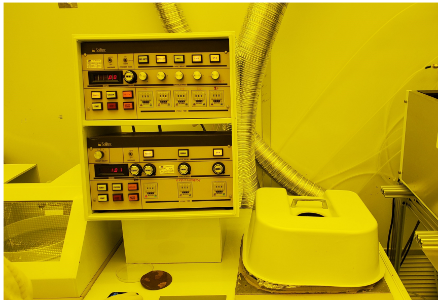
Figure 5.2: The machine used to spin SU-8 at 600 and 1000 rpm.
