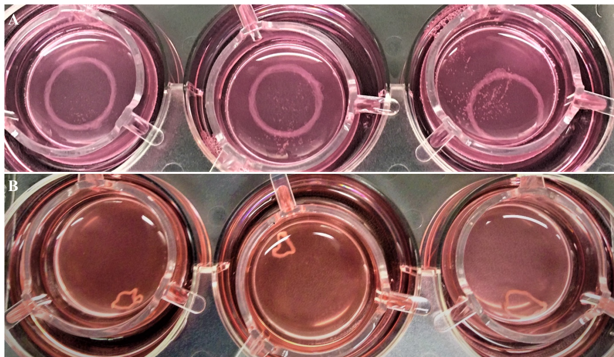
Figure 3.09. Evolution of 2691MA HASM cells printed with 0.75% alginate (100µM RGD-alginate + 0.25% SLG-20) + 2mg/mL collagen. (A) After printing. (B) After 7 days.
