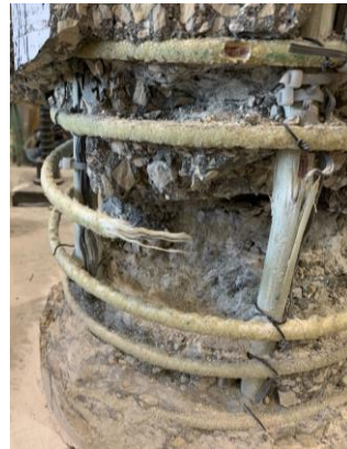
(b) Close-up view for bar and spiral failure – specimen GH-0.2-50.
