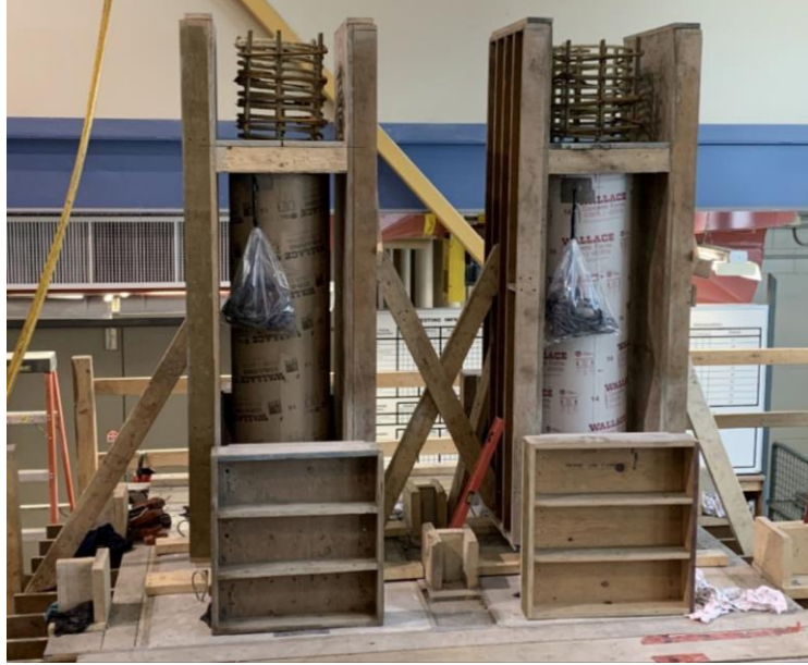
(b) Columns of the GFRP-RC specimens G6 and G7 ready for casting
