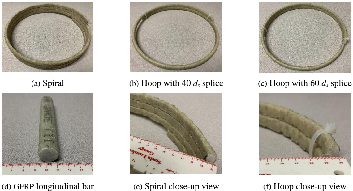
Figure 4.1: Samples of GFRP transverse reinforcement (dimensions in mm)
