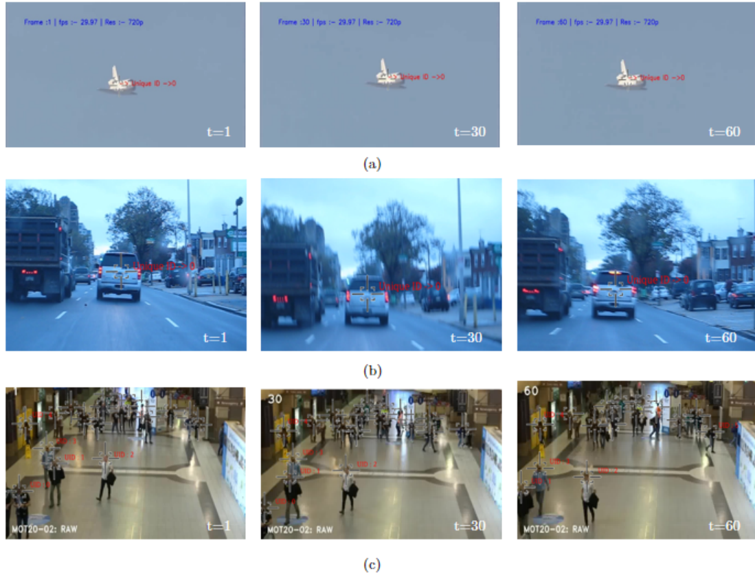
Figure 42: Results are being recorded over a few frames. (a) tracking result from a random Youtube video sequence, (b) tracking results from VOT-ST2020 training data, (c) tracking results from MOT20 training data. At each sequence, unique ids displayed maximum up to four objects. For more than 60 frames, these identities are tracked individually.
