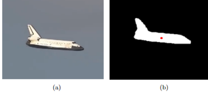
Figure 12: Centroid of a binary mask. (a) input frame (b) shape mask with the centroid (red)
