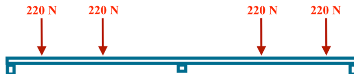
Figure 37: Load case for 0.3G braking event
