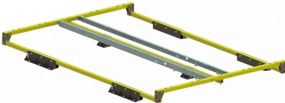
Figure 71: CNG rack without walkway
