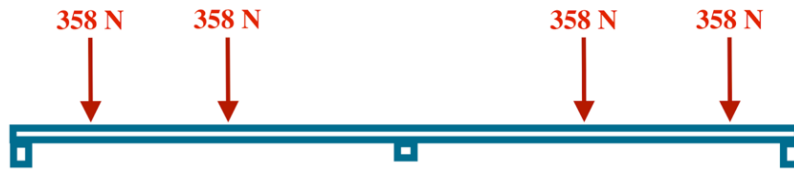
Figure 4: Front view of the front beam
