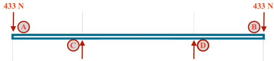
Figure 8: Free body diagram (FBD) of the side beam.
