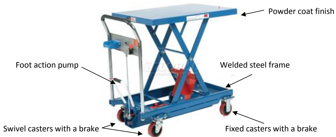
Figure 9: The Global Industrial lift cart, the typical lift cart on the market [5]
