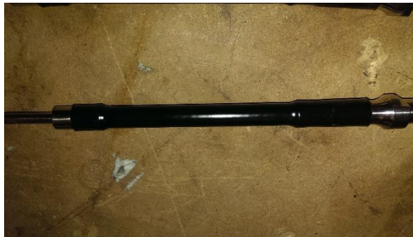
Figure 4: Flexible surgical drill bit with heat shrink tubing after heat addition
