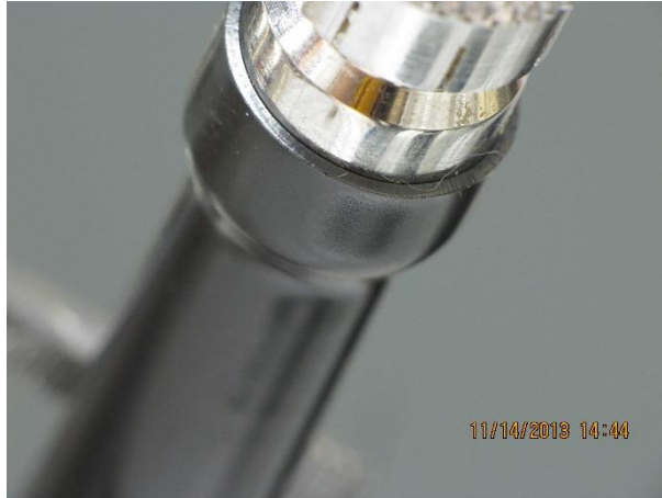
Figure 13: Flexible drill bit with heat shrink tubing shrunk onto the drill bit
