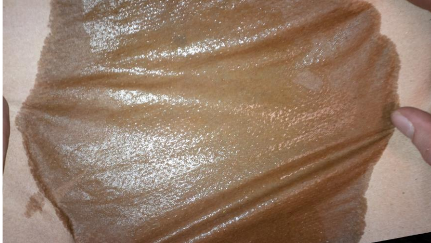
Figure 9: Filter after water from testing was poured through it
