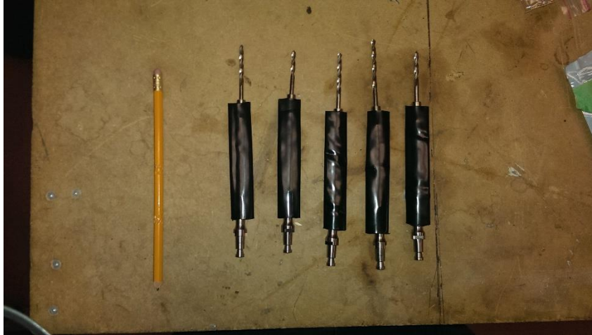
Figure 3: Flexible surgical drill bits with heat shrink tubing prior to heat addition
