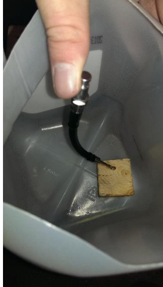
Figure 5: Wooden block retained keeping drill bit at an angle
