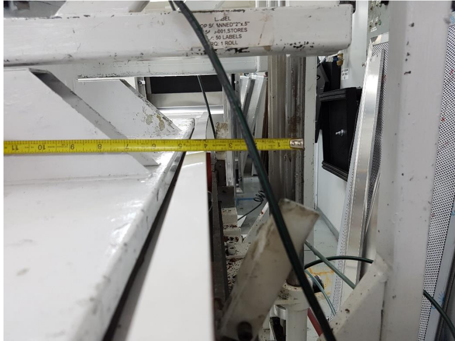
Figure A-2: Clearance around the back of the air diffuser and the test rig [4].
