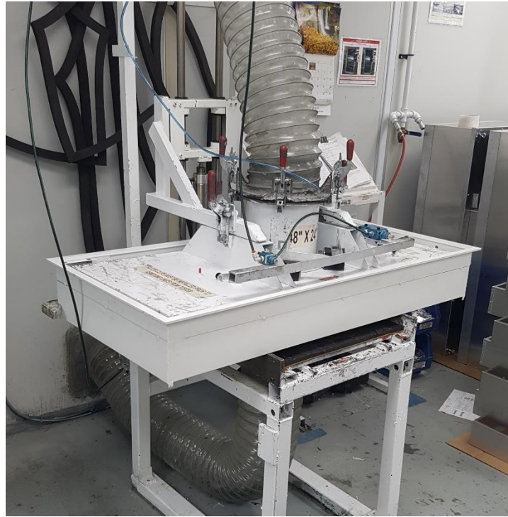
Figure 2: The test rig and HEPA filter diffuser assembly [2].
