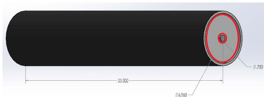
Figure E-83: Top Roller Shell and Shaft weld area [7].
