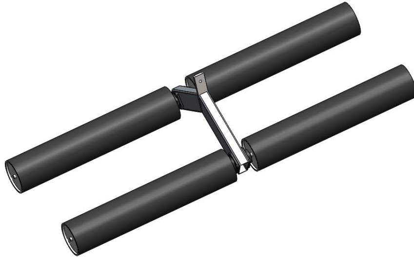
Figure 4-9: Back side isometric view of the top roller subassembly [9].
