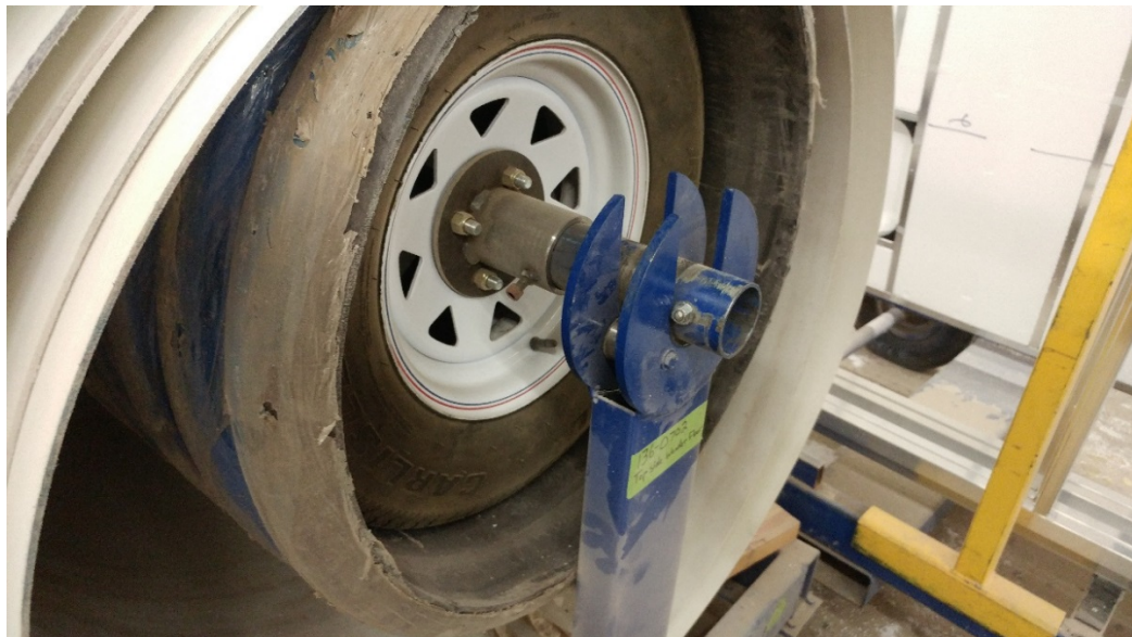
Figure 1-2: Vertical slots used to secure shaft [5].
