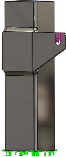
Figure E-94: Safety Bracket weld FEA boundary conditions [3].
