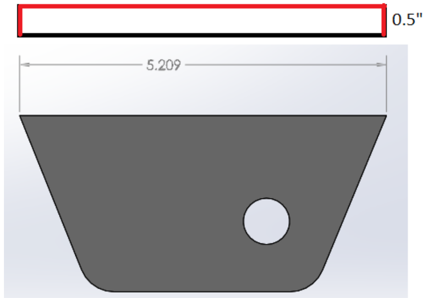
Figure E-86: Swinging Arm Top Bracket weld area [7].
