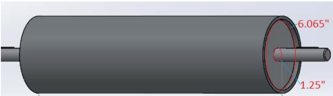
Figure E-90: Bottom Rollers Shell and Shaft weld area [7].
