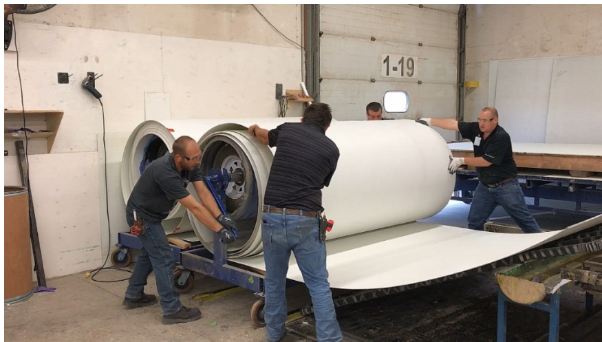
Figure 1-1: Material recoiling process requiring four workers [4].
