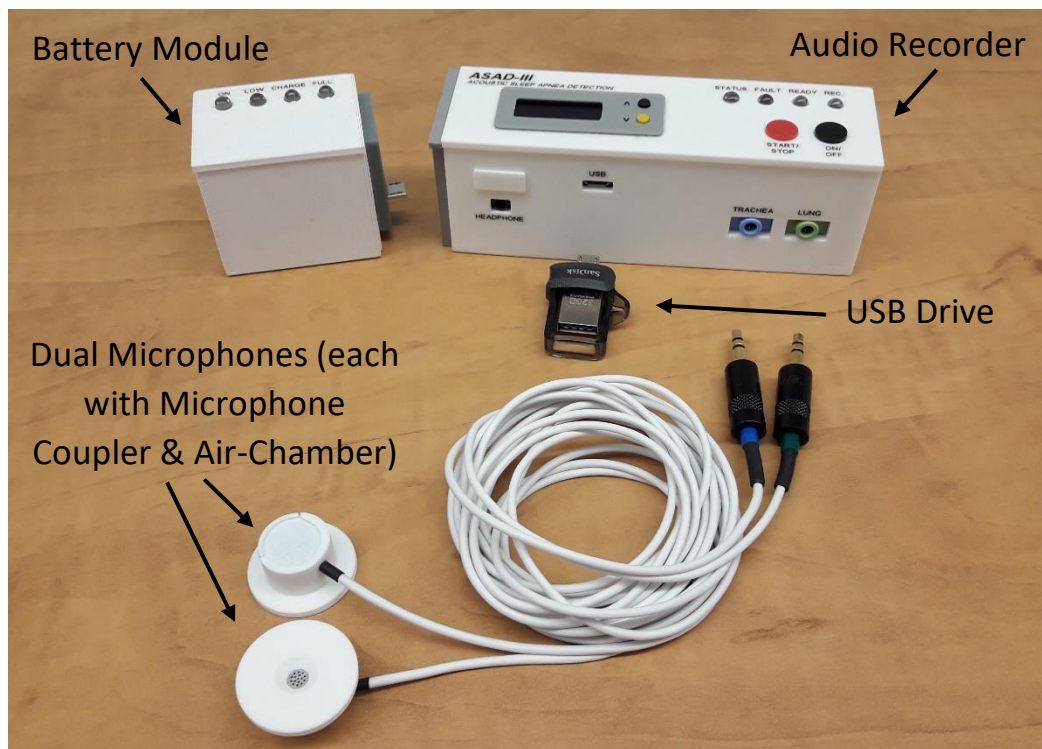
Figure 2.1. ASAD-III (Acoustic Sleep Apnea Detection, version 3) full system with components labelled.
