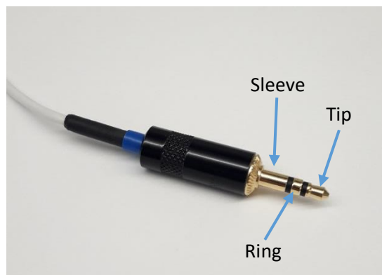
Figure 3.14. TRS (stereo) 3.5 mm plug with connections shown.
