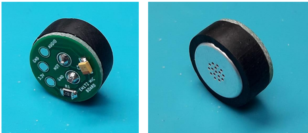
Figure 4.8. Primo EM172 microphone with Microphone Driver Circuit PCB attached. Left shows the back/side profile view, where right shows the front/side profile view. Note: rubber isolator ring (the use of which described by Chapter 5 of this report) is shown around microphone.
