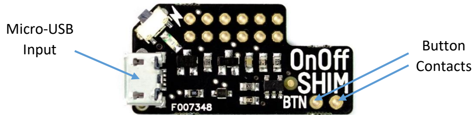
Figure 3.25. OnOff SHIM shown in original, as purchased configuration. Source: Adapted from [48].
