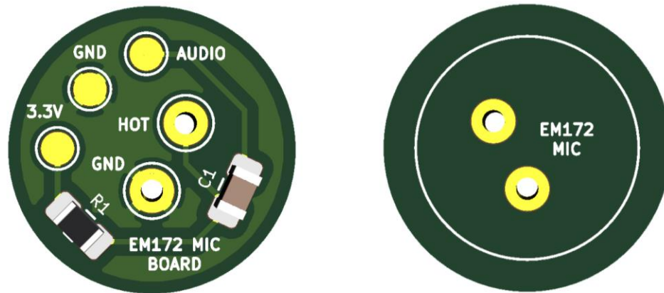
Figure 4.7. Custom designed printed circuit board (PCB) to implement the Microphone Driver Circuit. Front view (left) and back-side view (right).
