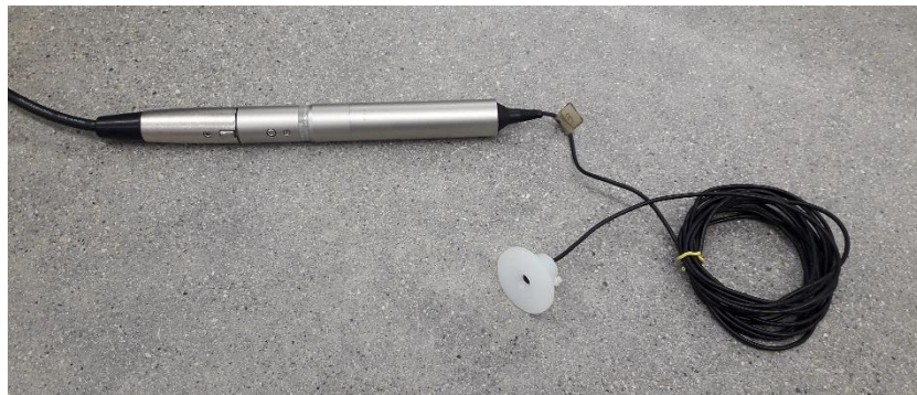
Figure 1.1. Sony ECM-77B electret condenser microphone; silver cylinder contains the battery and other related circuitry to power microphone. Microphone element shown inserted to custom Microphone Coupler.
