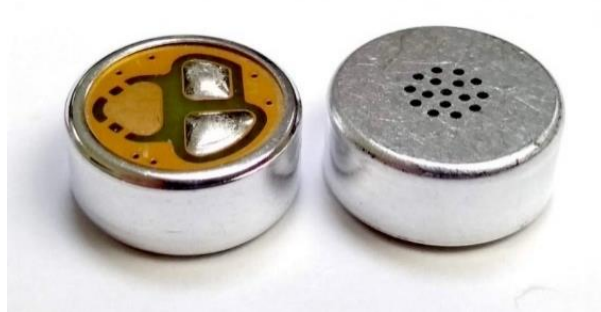
Figure 4.5. Primo EM172 electret condenser microphone backside (left) and front (right) shown. Source: [51]
