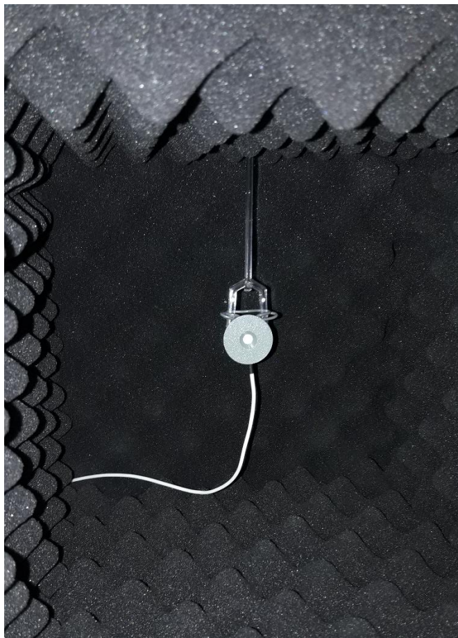
Figure 8.10. Microphone being tested placed inside the Microphone Isolation Box.
