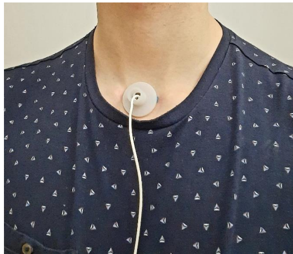
Figure 5.1. Revision 1 design of the Microphone Coupler shown affixed at the suprasternal notch for recording tracheal sounds.
