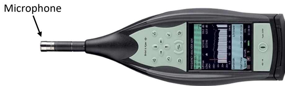
Figure 3.42. Brüel & Kjær (B&K) model Type 2250-S sound level meter. Source: [53]
