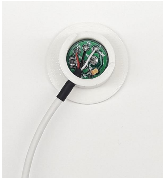
Figure 4.9. Microphone Coupler with protective cap removed showing the internal connections to the Microphone Driver Circuit PCB attached.
