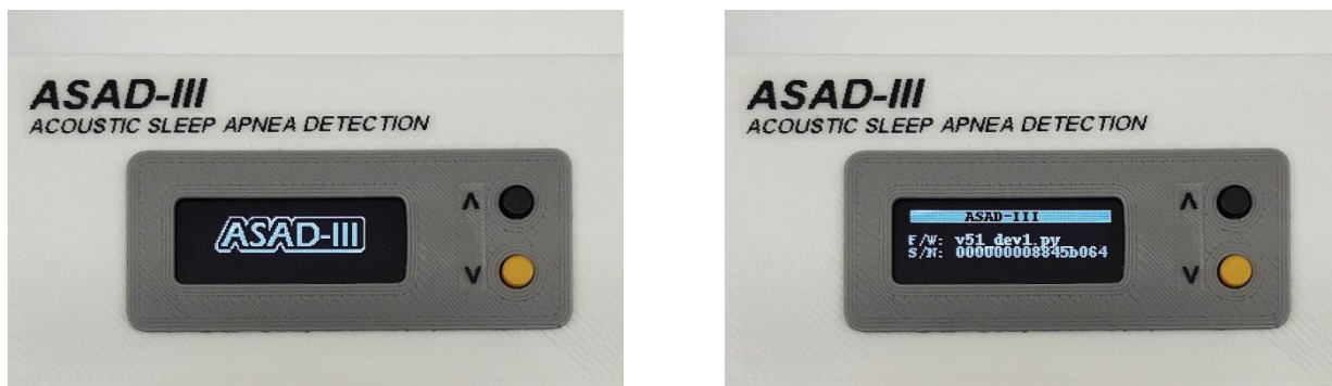
Figure 3.34. Audio Recorder shown powered on demonstrating the information presented by OLED display on start-up and loading of the OS. Left shows the splash screen, right shows the device information screen.
