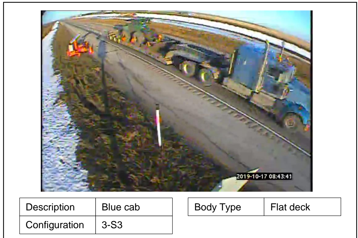
Figure 35 - Screenshot from camera installed at portable WIM system with accompanying information
