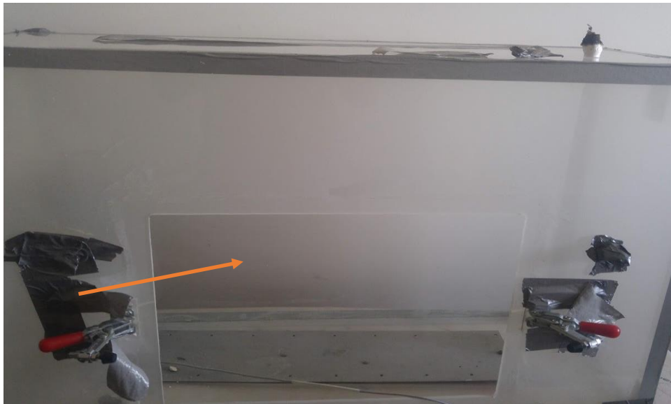
Fig. 4.11 Deposition of smoke particles on the chamber walls.
