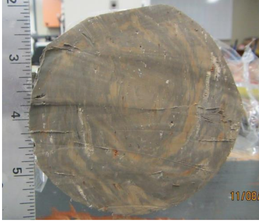
Figure A-B.12 WD clay foundation trimmed sample
