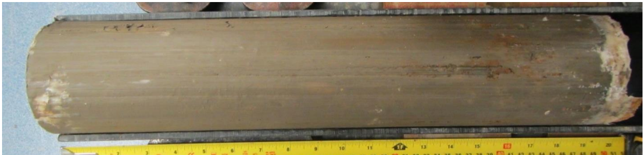
Figure A-B.3 CBMD clay core extruded Shelby tube sample
