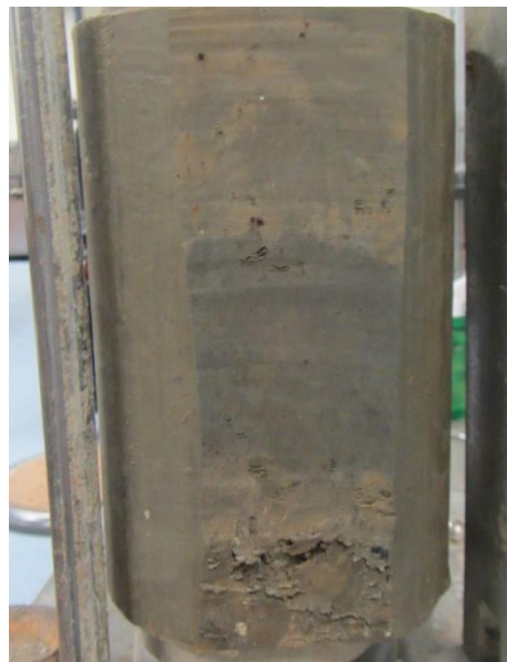
Figure A-B.11 WD clay core trimmed sample
