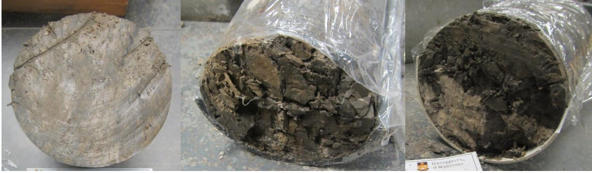
Figure 4.8 CBBD2 clay foundation samples
