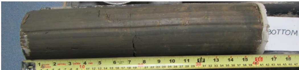
Figure 4.3 CBB2 clay foundation extruded Shelby tube sample
