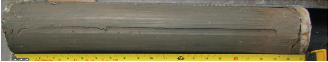
Figure A-B.1 CBBD4 clay core extruded Shelby tube sample
