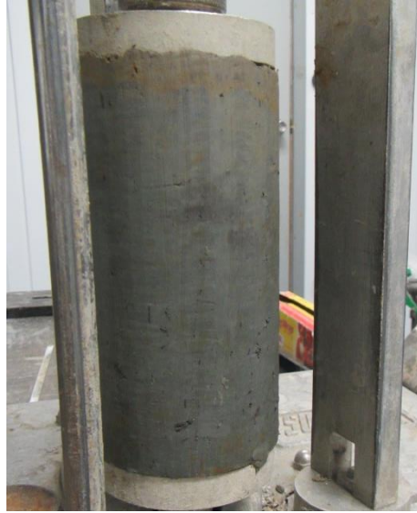
Figure A-B.10 CBBD4 clay foundation trimmed sample
