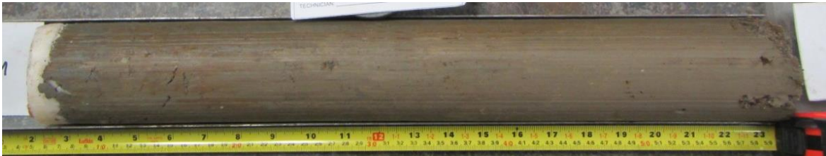
Figure 4.2 CBB2 clay blanket extruded Shelby tube sample
