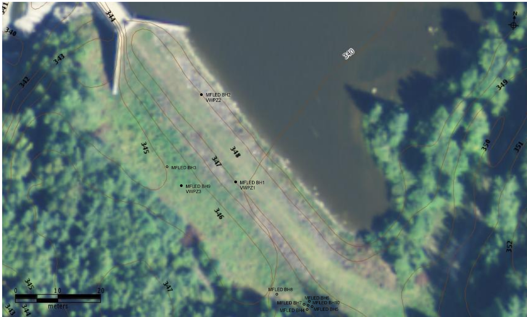
Figure 3.6 Approximated location of boreholes, test pits and installed vibrating wire piezometers in MFLED
