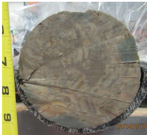
Figure A-B.16 MFLED clay core trimmed sample
