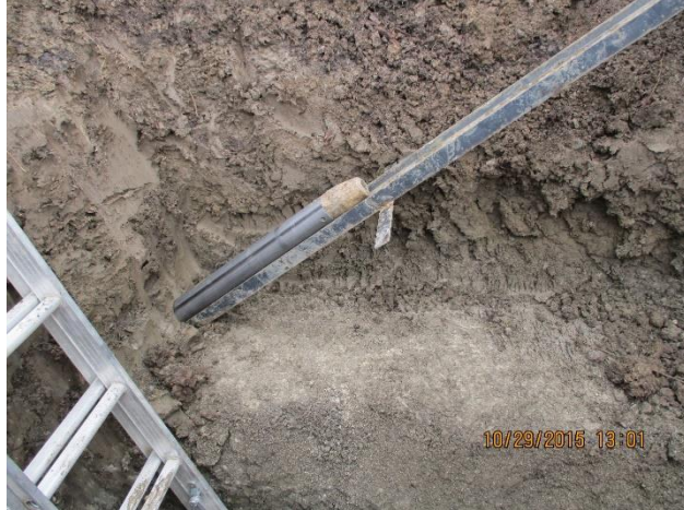
Figure 3.8 Collection of inclined samples in a CBBD2 test pit
