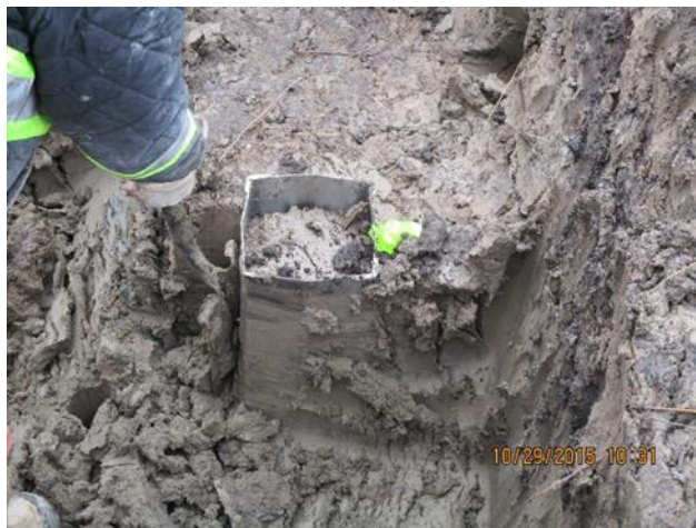
Figure 3.9 Samples obtained in a CBBD2 test pit by means of a block sampler
