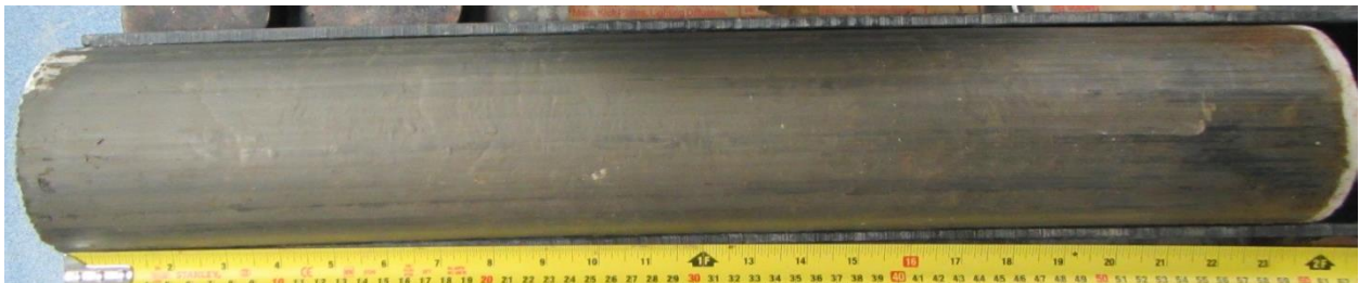
Figure A-B.4 WD clay core extruded Shelby tube sample
