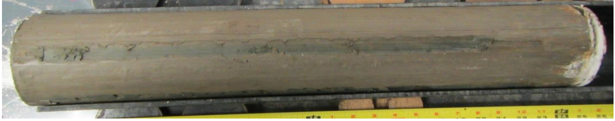
Figure A-B.9 MFLED clay core extruded Shelby tube sample
