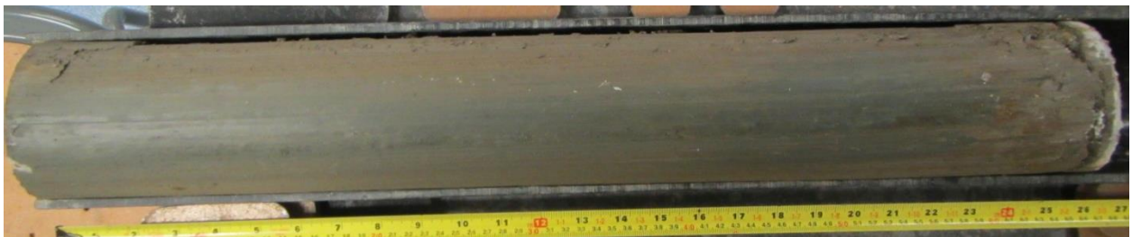
Figure A-B.8 MFRED clay core extruded Shelby tube sample
