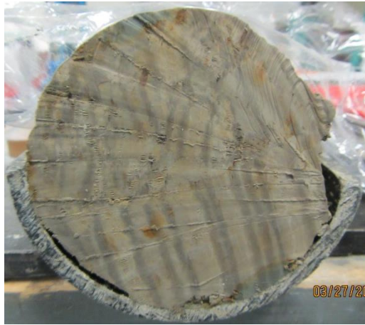
Figure A-B.15 MFRED clay core trimmed sample
