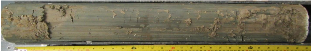
Figure A-B.7 EF clay foundation extruded Shelby tube sample
