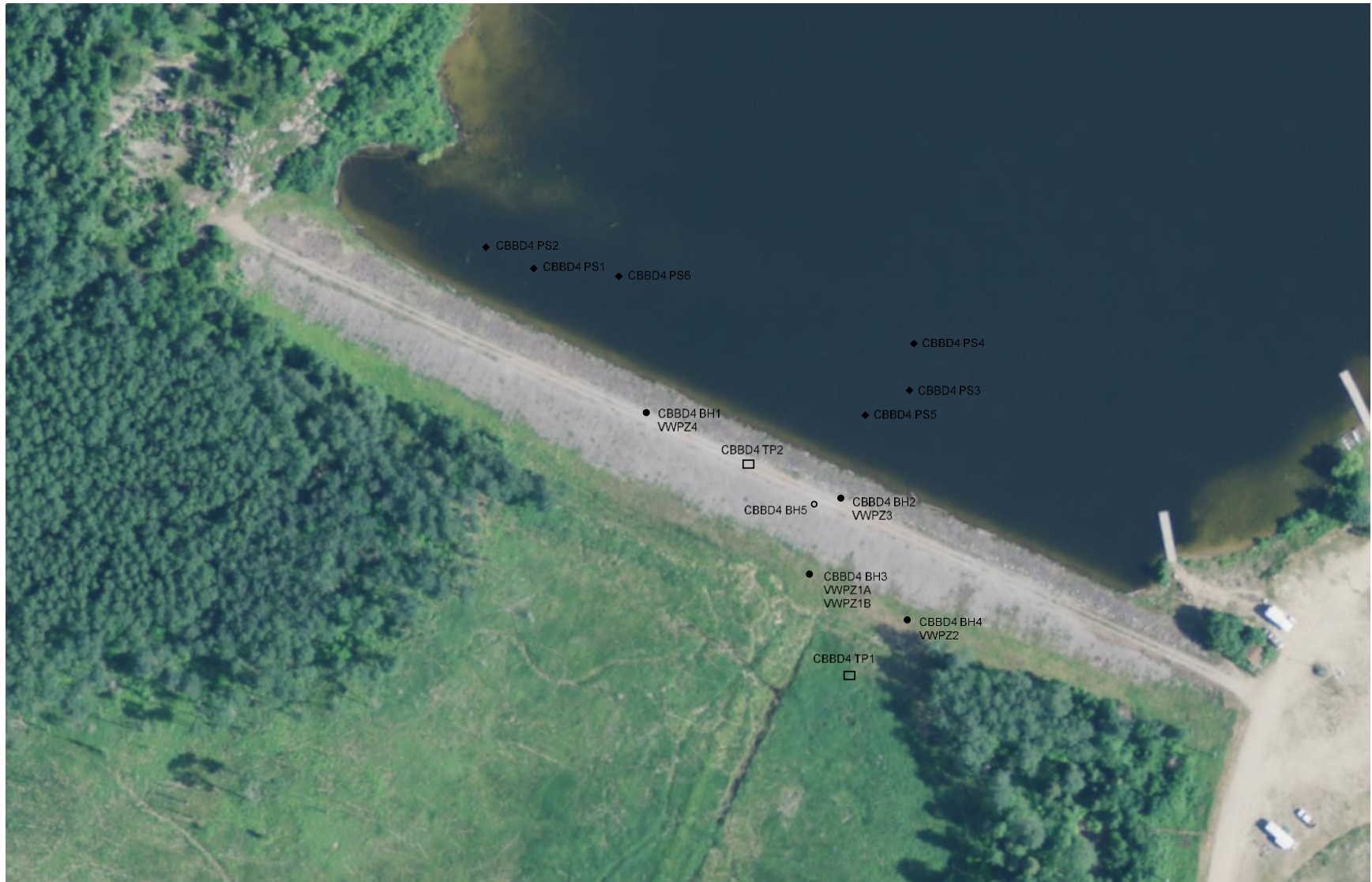
Figure 3.2 Approximated location of boreholes, test pits and installed vibrating wire piezometers in CBB4
