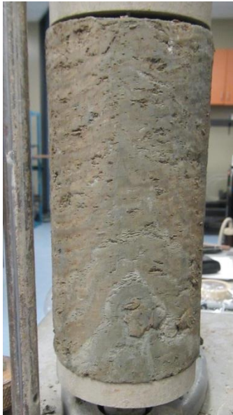
Figure A-B.14 EF clay foundation trimmed sample
