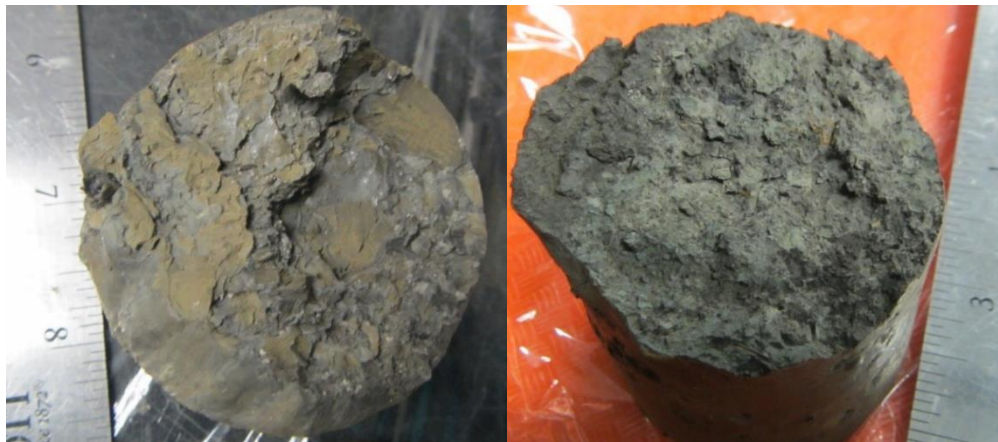
Figure 4.33 CBB2 clay blanket post-CIU Triaxial Test test samples
