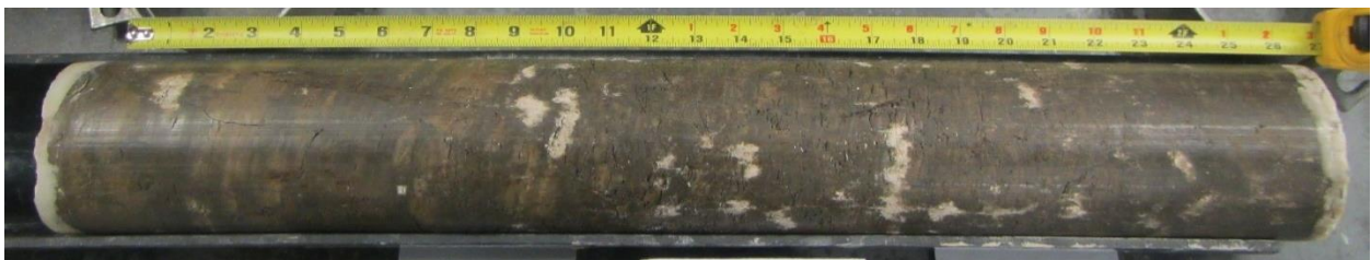
Figure 4.4 CBB2 clay foundation sample at location further away from CBB2
