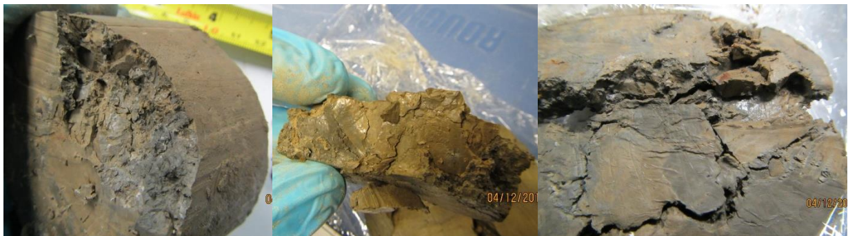
Figure 4.7 Fissures and polished surfaces observed in clay blanket samples
