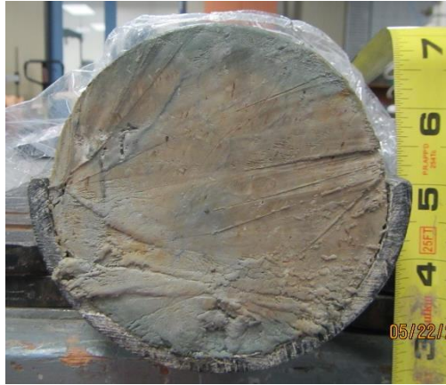
Figure A-B.13 EF clay core trimmed sample
