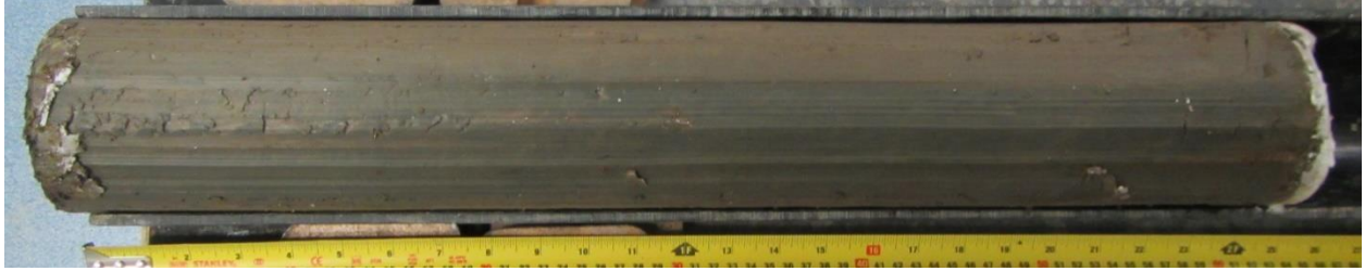
Figure A-B.5 WD clay foundation extruded Shelby tube sample
