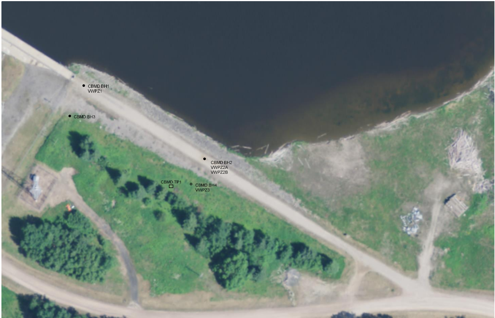
Figure 3.3 Approximated location of boreholes, test pits and installed vibrating wire piezometers in CBMD
