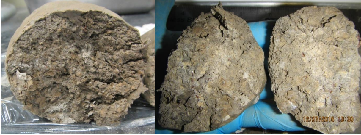
Figure 4.34 CBB2 clay foundation post-CIU Triaxial test samples
