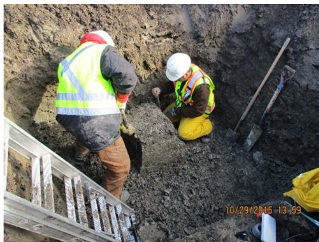
Figure 3.10 Conventional soil block sampling in a CBBD2 test pit
