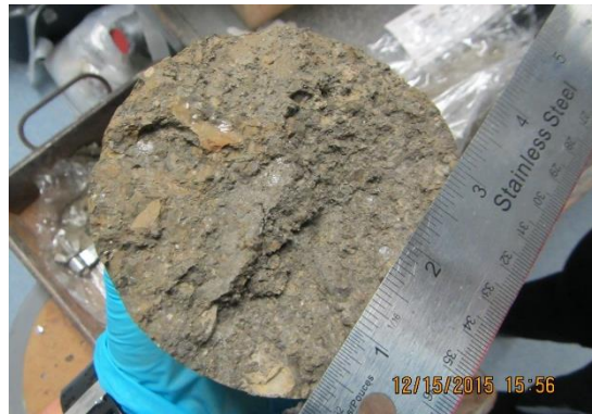
Figure 4.6 Polished surfaces observed in CBB2 clay core sample
