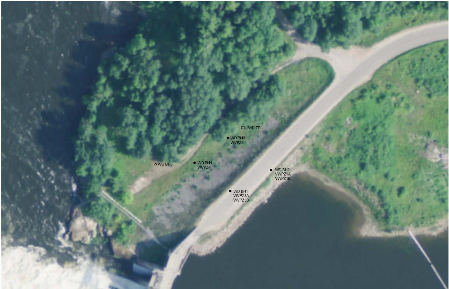
Figure 3.4 Approximated location of boreholes, test pits and installed vibrating wire piezometers in WD
