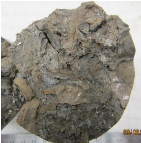
Figure 4.35 CBB4 clay core post-CIU Triaxial test samples
