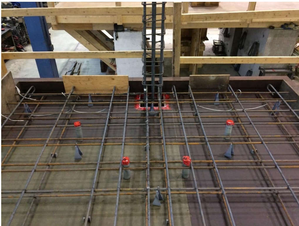
Figure 3.18: Specimen 1 (steel-RC) before casting
