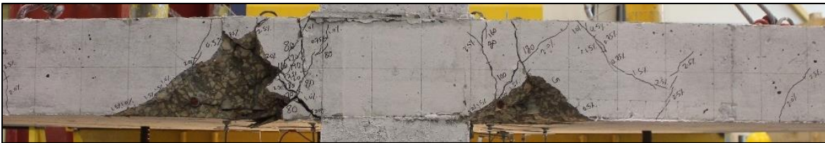
b) Slab free edge after 2.50% drift ratio
