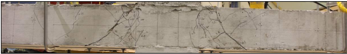
b) Slab free edge after 2.50% drift ratio
