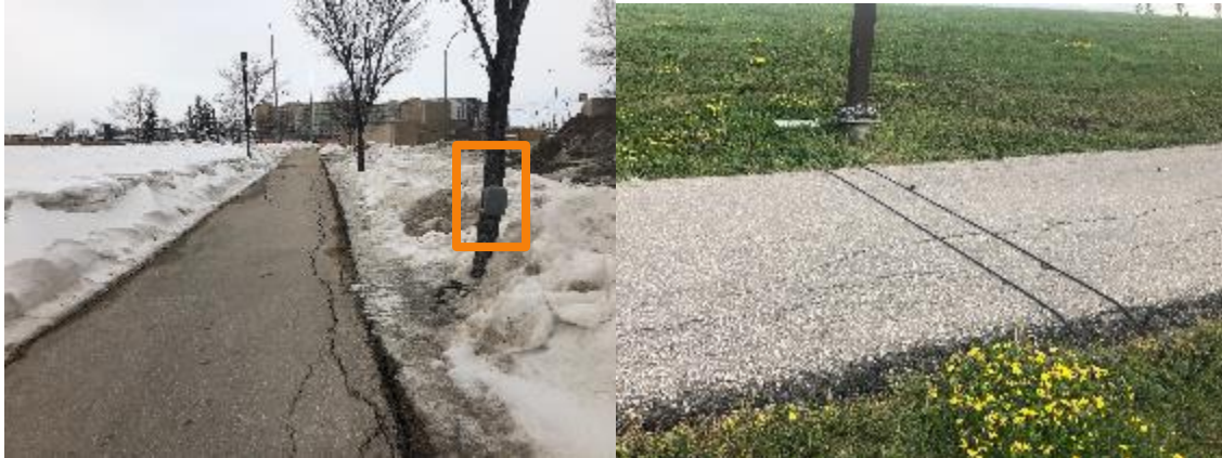
Figure 3.19: Chancellor Matheson ground view on south pathway (left: passive infrared sensor facing west; right: pneumatic tubes)
