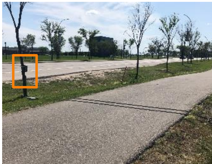
Figure 3.18: Chancellor Matheson ground view on north pathway facing west (passive infrared and pneumatic tubes)
