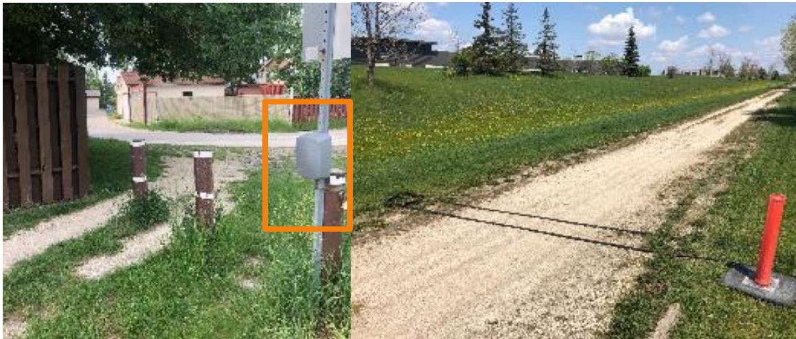
Figure 3.16: Smartpark ground view (left: passive infrared sensor facing west; right: pneumatic tubes facing east)
