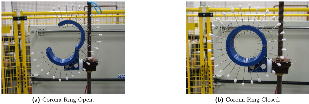
Fig. 4.5: Corona ring of needles used for applying non-contact space charge.
