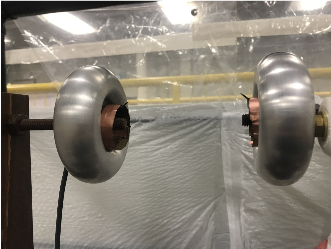
Fig. 5.1: Air insulated test unit
