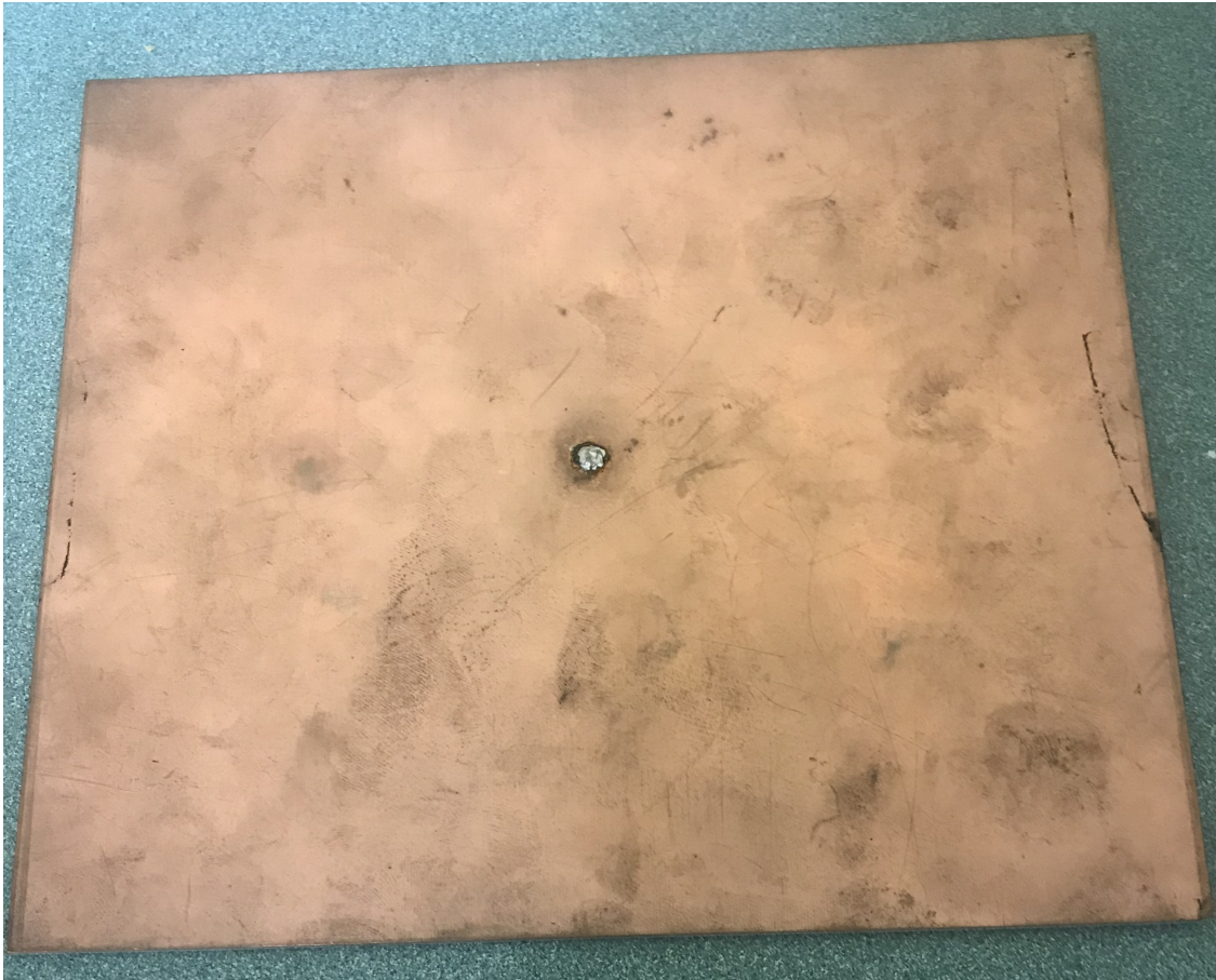
Fig. A.3: Parallel plate electric field sensor used for PD detection.
