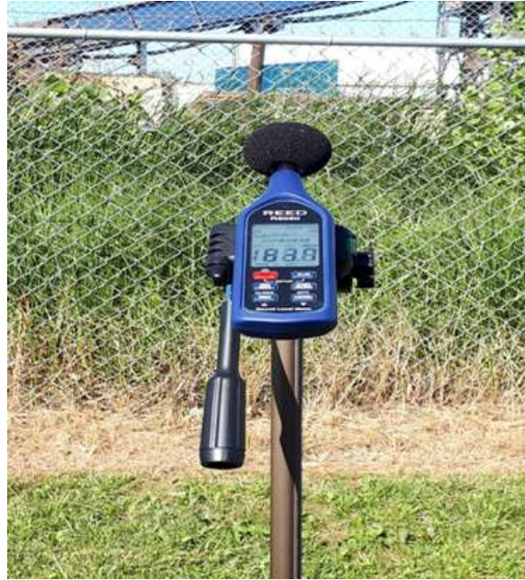
Fig. 3.5 REED digital logging sound level meter installed for logging noise levels in dBA during scrap metal shredding in Mission Industrial Area, Winnipeg (July, 2018).
