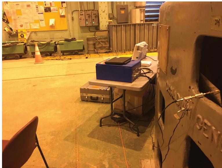
Fig. 6.5: Antenna placed in an upper stator frame window. The conditioning circuit is connected to the antenna and the oscilloscope is on the table next to the stator frame.
