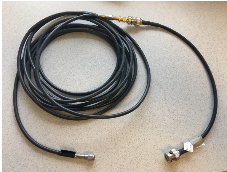
Fig. 4.5: RG-58 cable assembly that connects to the antenna (at male SMA end) to the oscilloscope (male BNC end).
