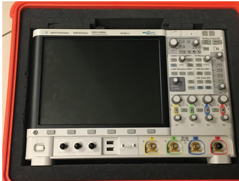
Fig. 4.4: High speed oscilloscope used for UHF PD measurements.
