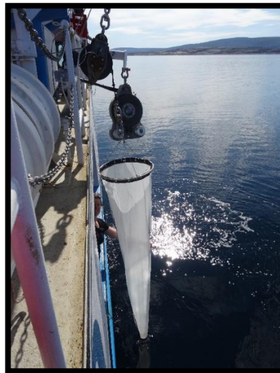
Figure 8 A zooplankton net was lowered from the starboard side of the Nuliajuk using the scientific winch.
