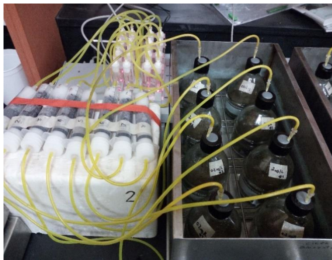
Figure 2.3 BMP assay setup in the water bath and respirometer
