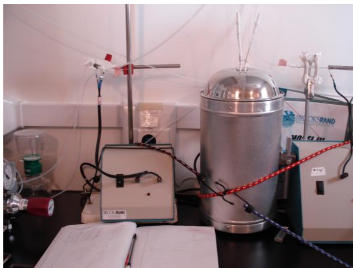
Figure 1: Trap and column to separate the organic mercury species
