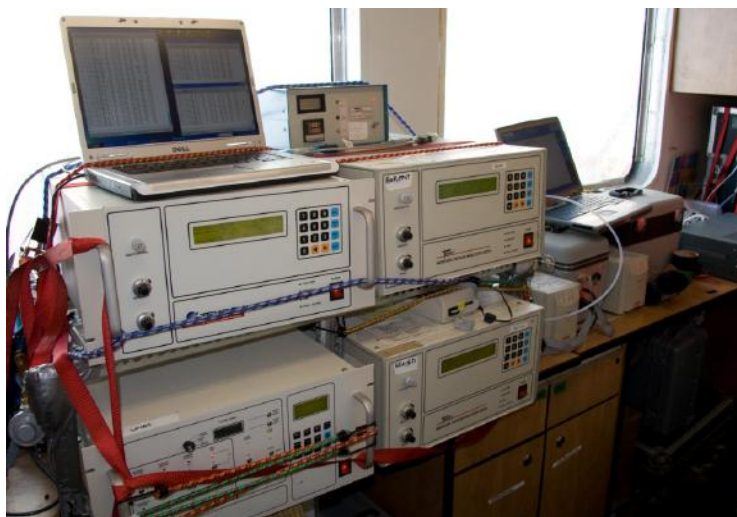
Figure 7: Tekran 2537 ambient mercury vapor analyzers with pump unit
