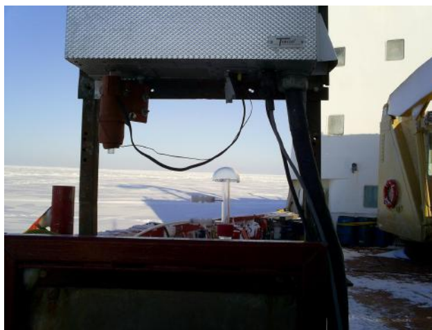
Figure 1. Sampling head for the Arctic Pyrolyser (right side) and for the Mercury speciation system (left side)
