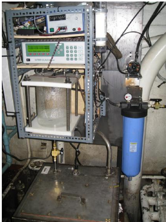
Figure 1.4: The on-track pCO 2 system located in the engine room of the Amundsen. The equilibration chamber is the clear cylinder (left bottom) and the gas analyzer is the box with the digital display.
