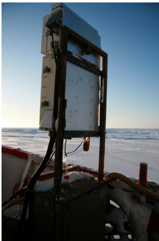
Figure 6: Tekran 1130/1135 speciation unit with 1105 pyrolysis unit
