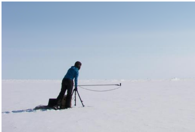
Fig. 3. Setting up the ASD to collect downwelling irradiance.
