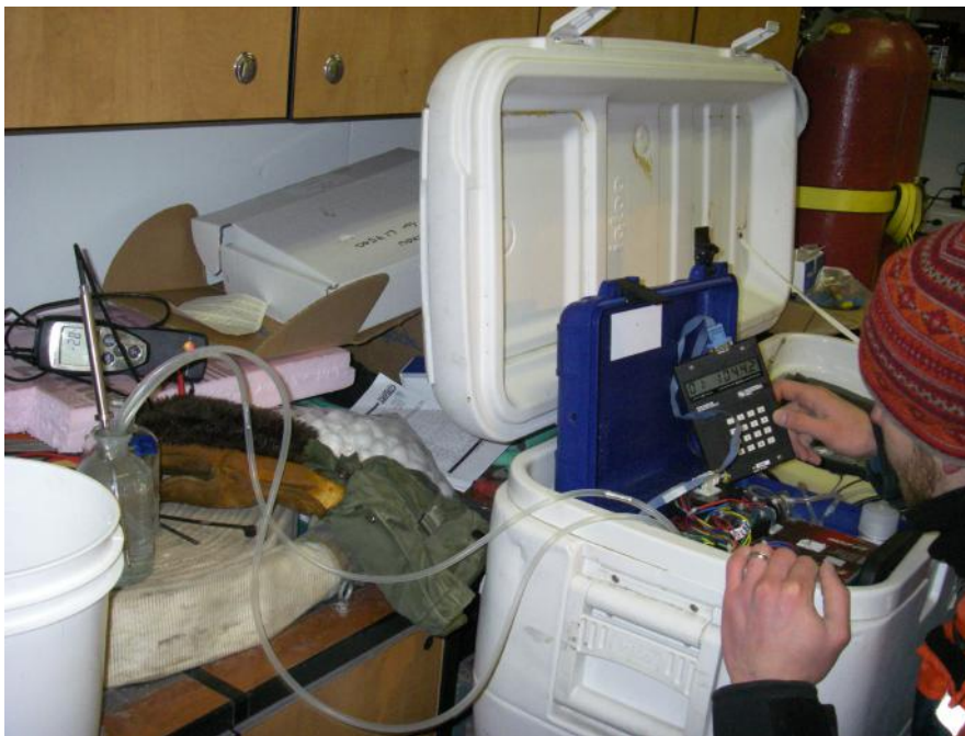
Figure 2.4: Sampling set up for brine pCO 2 . In later instances the bottle was kept at a lower temperature by working in an ice bath, or a cool room. The bottle top was capped with parafilm to limit gas exchange.
