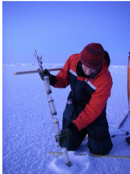
Figure 2.1: Deployment of a peeper array into an auger hole drilled through the ice to the ocean.
