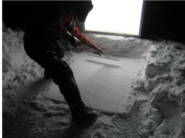
Fig 2.4. The experiment to measure the attenuation coefficient of the light through snow layers of different thicknesses.
