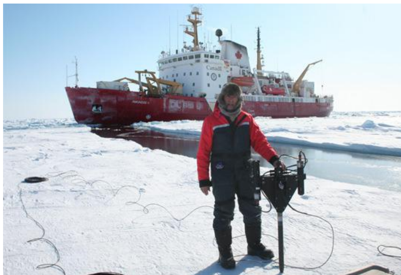
Figure 8. Hyper OCR about to be deployed at dive location
