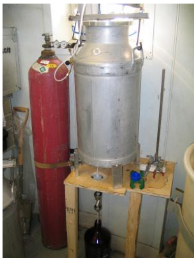
Figure 3. Snow-can meltwater extraction
