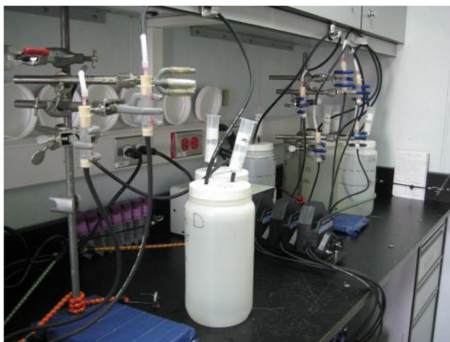
Filtration of water through WAX cartridge with additional cartridge acting as an air filter.
