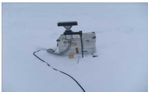
Figure 1. Hi-vol air sampler deployed on the ice at CFL station D43
