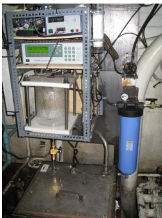
Figure 2: The on-track pCO 2 system located in the engine room of the Amundsen. The equilibration chamber is the clear cylinder (left bottom) and the gas analyzer is the box with the digital display.
