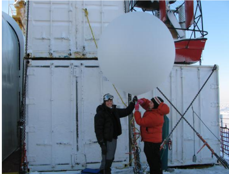
Figure 4. Attaching a radiosonde to a balloon for an atmospheric profile.
