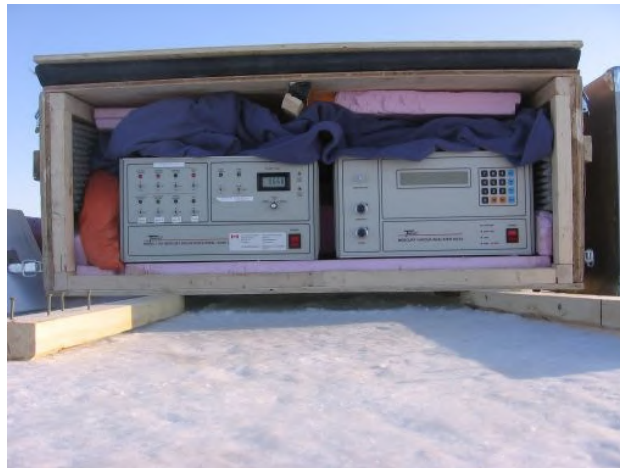
Figure 3: pump and atomic fluorescence instrument
