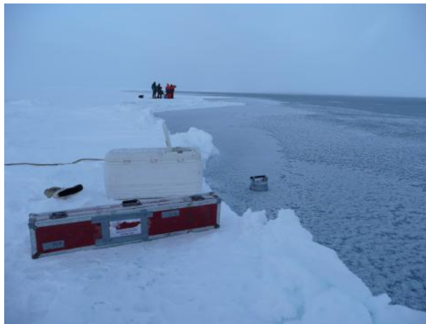
Figure 2.1: Deployment of the flux chamber. Gas analyzer is located in the white cooler.
