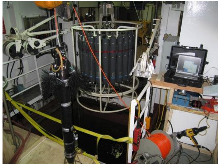
Figure 1: VMP installation in the moonpool area.
