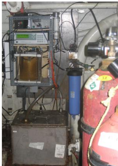
Figure 4: The on-track p\text{CO}_2 system located in the engine room of the Amundsen. The equilibration chamber is the clear cylinder. Seawater is filtered in the blue cylinder before entering the chamber. The gas analyzer is the box with the digital display. To the right of it, the container of desiccant is seen. The tanks with \text{N}_2 and \text{CO}_2 are seen in the foreground.
