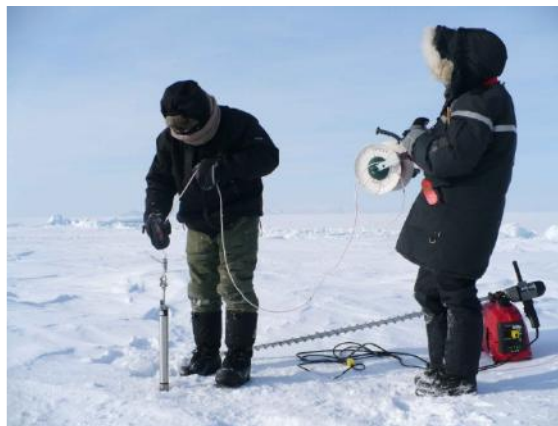
Figure 3. A CTD and PAR profile through the snow and ice
