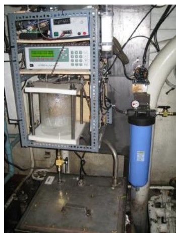
Fig. 4. The on-track p\text{CO}_2 system located in the engine room of the Amundsen.
