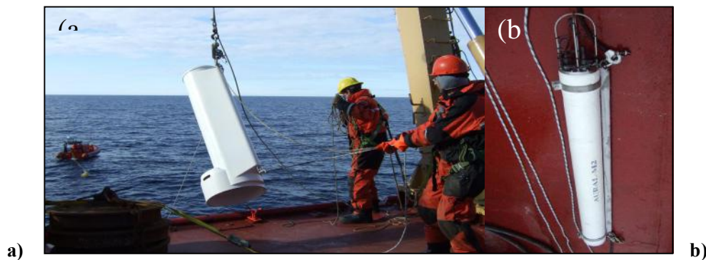
Figure 3: Instruments on the moorings: (a) Sediment trap Technicap PPS 3/3 24-cups being deployed at CA04; b) Passive acoustic hydrophone AURAL M2
