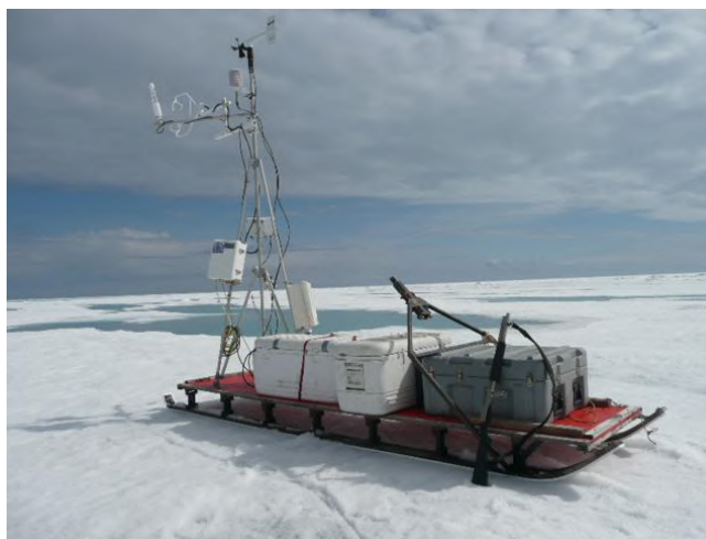
Figure 2: The portable ice meteorology/flux station. For this deployment, the closed path sensor and radiation sensors were not included. They were included in later deployments (see Table 2).
