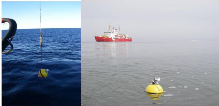
Fig. 7. Meteorological Ocean Buoy (MOB) deployment by line (left) and data acquisition (right).
