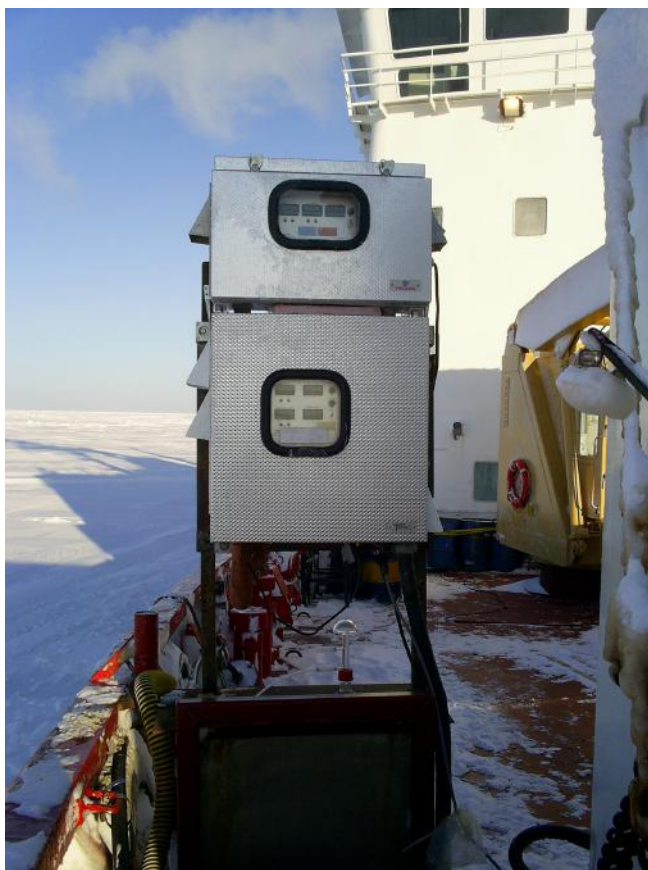
Figure 3. Sampling systems for the Arctic Pyrolyser (bottom) and the Mercury Speciation system (top).
