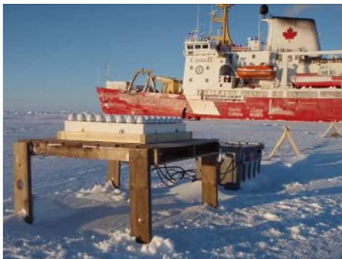
Fig. 6. The Scintec MFAS sodar next to the ship on 9 March 2008
