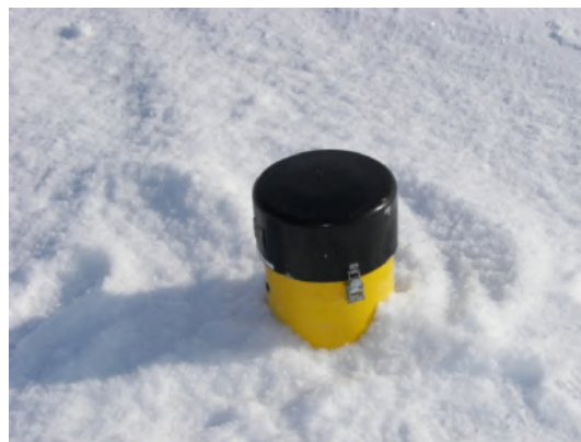
Figure 11. Ice motion beacon installed in a first-year ice floe.
