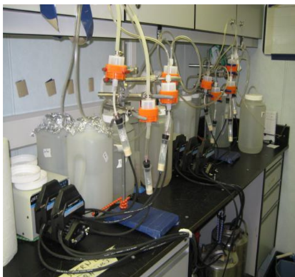
HCH water filtration (Aft chemistry lab)
