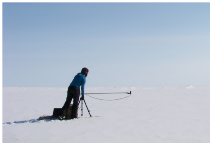
Figure 5. Setting up the ASD to collect downwelling irradiance.
