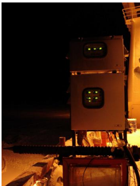
Tekran atmospheric mercury system on the foredeck of the ship.
