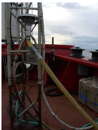
Air sampler for perfluorinated compounds
