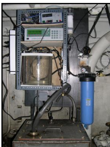
Figure 4. Sea water pCO 2 flow-through system in the forward engine room.
