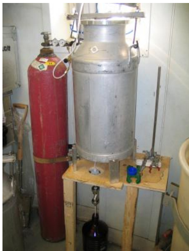
Figure 3. Snow-can meltwater extraction
