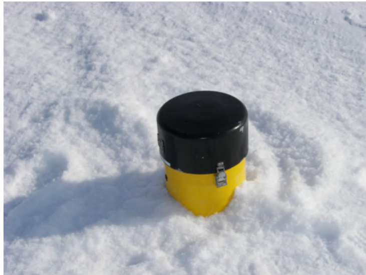
Figure 5. Ice motion beacon installed in a first-year ice floe.
