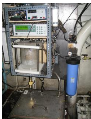
Figure 1.6: The on-track pCO 2 system located in the engine room of the Amundsen. The equilibration chamber is the clear cylinder (left bottom) and the gas analyzer is the box with the digital display.
