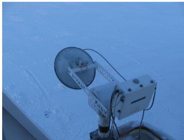
Fig. 1. Scatterometer mounted on the starboard side of the ship and overlooking the sample area that was previously marked out using flags.
