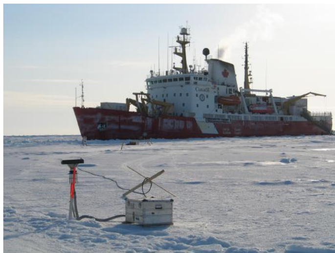
Figure 1. Hi-vol air sampler deployed on the ice at CFL station 31
