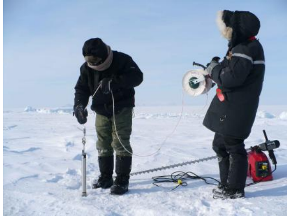
Figure 7. A CTD and PAR profile through the snow and ice
