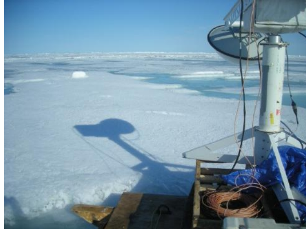
Figure 1. View from behind the ground-based scatterometer (foreground right) and field of view over a snow patch on melt ponded first-year sea ice.
