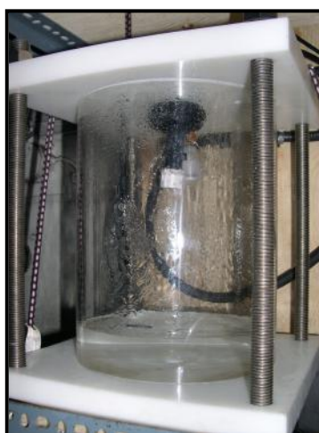
Figure 4. Sea water pCO 2 flow-through system in the forward engine room.
