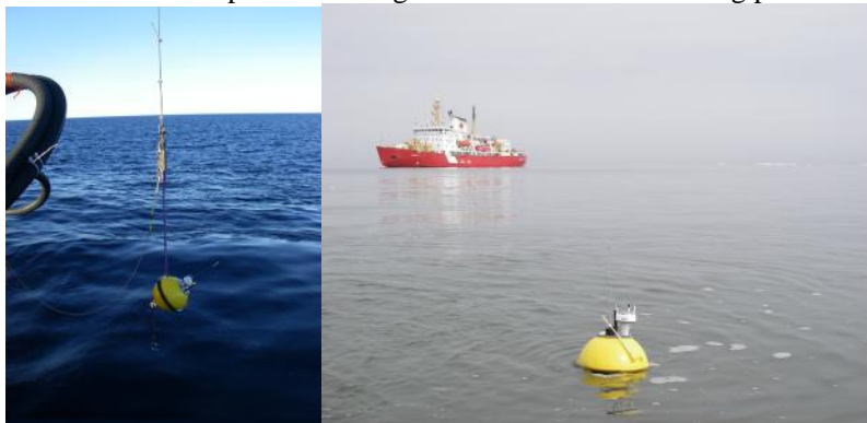
Fig. 2. Meteorological Ocean Buoy (MOB) deployment by line (left) and data acquisition (right).
