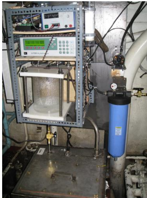
Figure 1.4: The on-track p\text{CO}_2 system located in the engine room of the Amundsen. The equilibration chamber is the clear cylinder (left bottom) and the gas analyzer is the box with the digital display.
