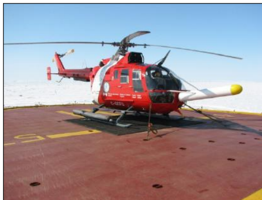
Figure 9. EM induction system mounted on the front of the helicopter.
