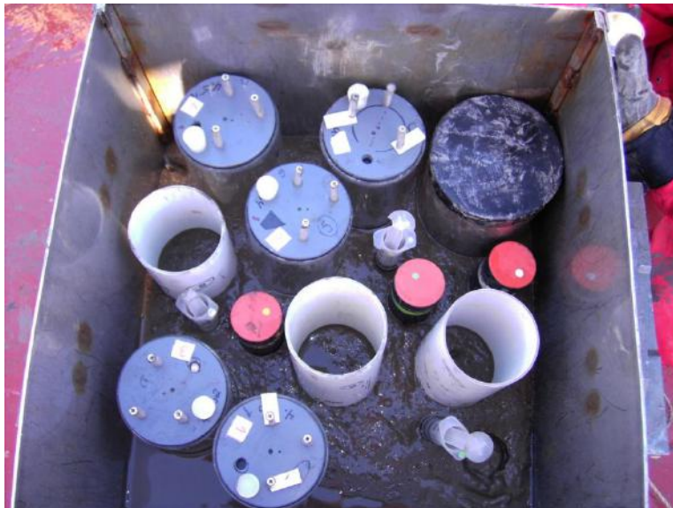
Fig. 1: Boxcore with SOD/Nutrient cores (grey), bioturbation cores (white), Chlorophyll a cores (orange), CN cores (syringes), and a biomarker core (black).
