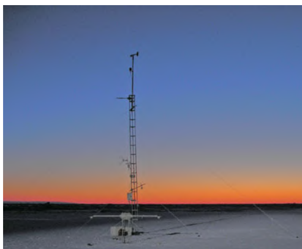
Fig. 2. Meteorological mast and heat flux tower at the ice station.
