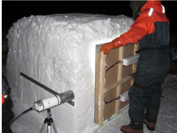
Fig 2.3. The experiment to measure the attenuation coefficient of the light through snow
