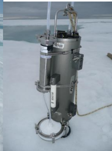
SeaStar high volume pump with XAD column and filter attached.
