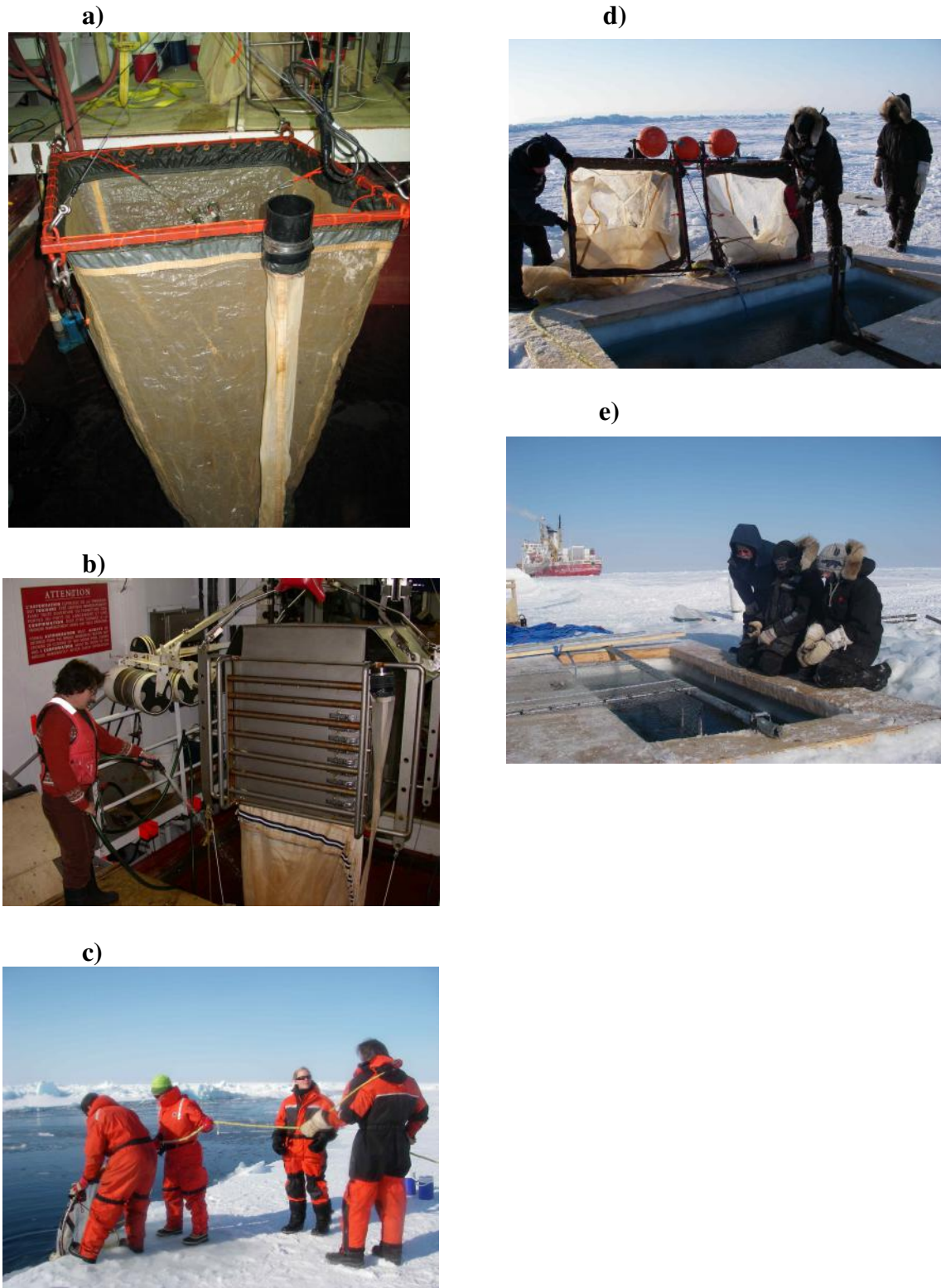
Figure 2. Zooplankton sampling gear used during CFL-Leg 7: a) 1-m 2 Square net and b) Hydrobios, both deployed from the moonpool, c) ring net, d) double net and e) gill net deployed from the ice.
