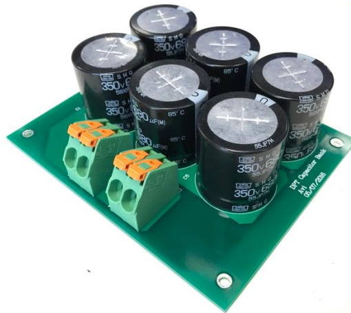
Figure 2.12 Image of DPT capacitor bank.
