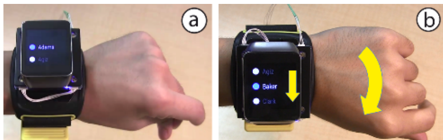
Figure 4.11: (a) User snaps to activate IMU function and (b) tilts the hand to scroll items.
