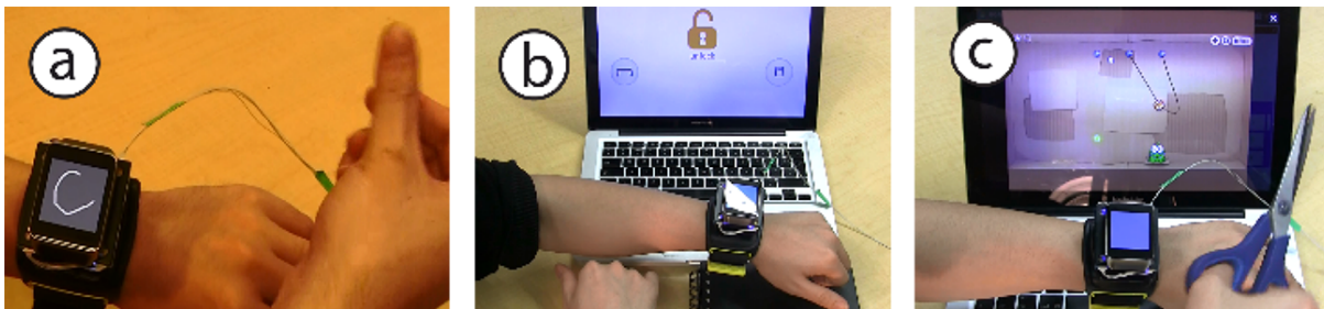
Figure 4.12: (a) A user sketches on the smartwatch with finger rubs. (b) The user unlocks the screen with a chain of acoustic signatures. (c) The user “cuts” the rope with a scissor in a game.
