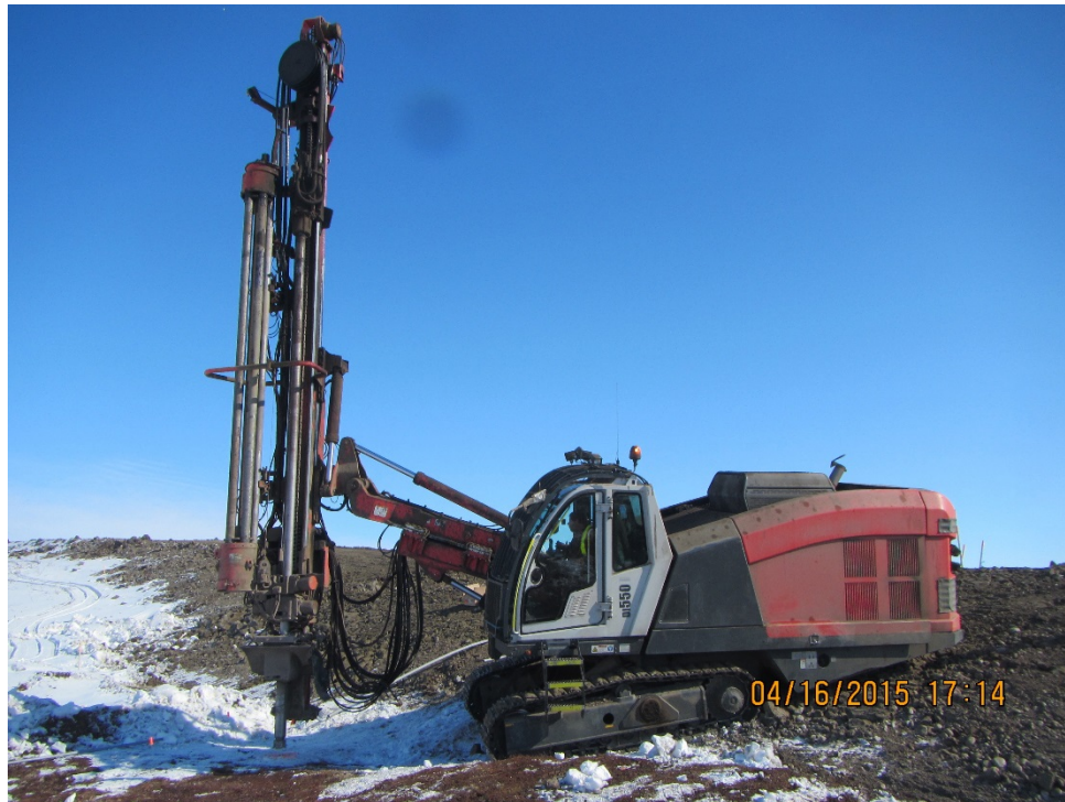
Photo 11: DTH drill rig used for drilling of holes for vertical SAA and vertical thermistor string installation
