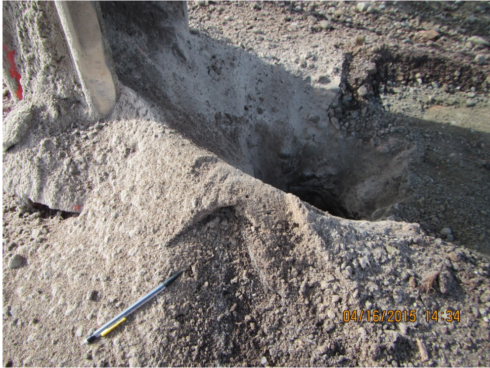
Photo 13: Materials adjacent to drill hole following DTH drilling
