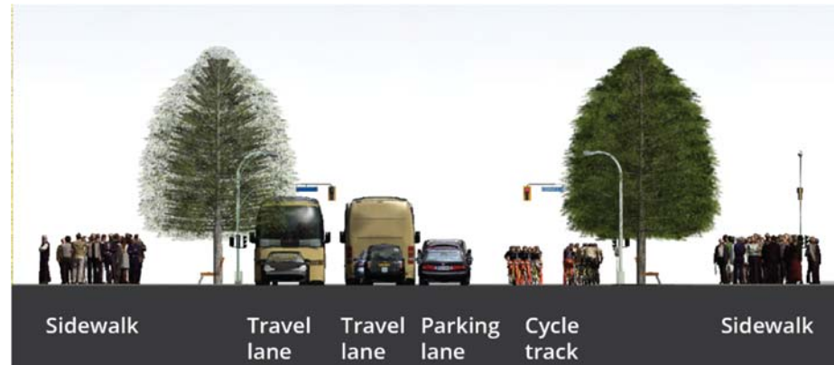
Figure B 16 – Section D-D – Regular Street. Adapted from Complete Streets by Esri Redlands & Esri Zurich, 2016. 1
