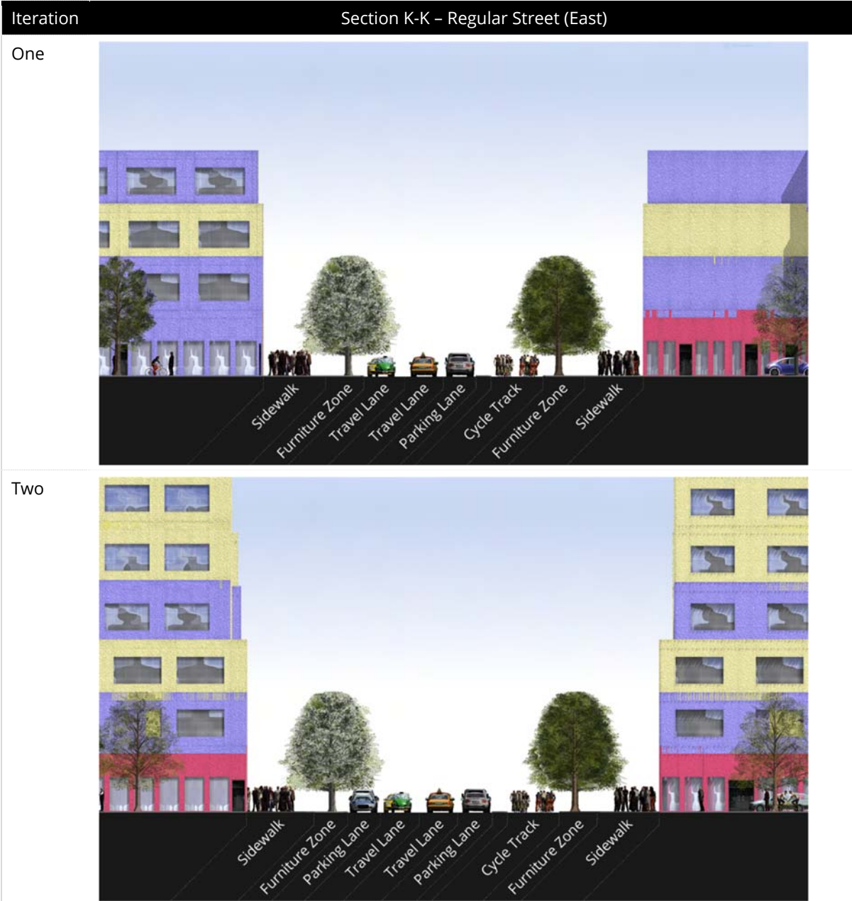
Figure C 39 – Tyne-Tees centre site iterations, Section K-K, regular street looking east. Adapted from: Complete Streets by Esri Redlands & Esri Zurich, 2016.
