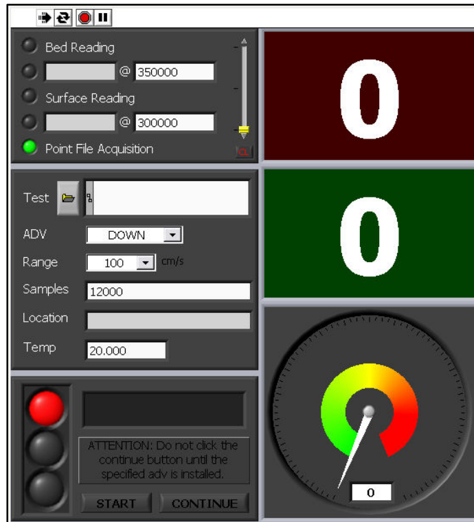
Figure 2.12 Front panel of LabVIEW program to control traversing mechanism
